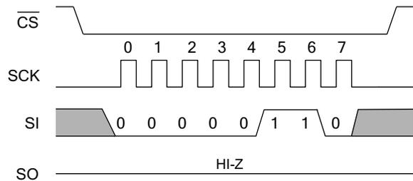
**WRDI - Reset Write Enable Latch**
