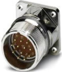
Device connector, front mounting, straight, Screw locking, M23, Number of positions: 17, Type of contact: Male connector, Crimp connection, Axial O-ring, 4xØ3,2, Shielded: Yes
