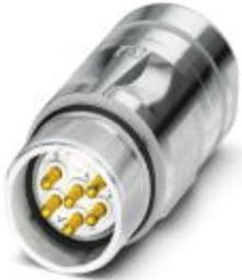
Coupling connector, straight, shielded: yes, SPEEDCON locking, M23, Number of positions: 6, Type of contact: Male connector, Solder connection, Cable diameter: 4 mm ... 6 mm
