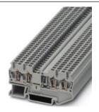
Component terminal block, Connection type: Spring-cage connection, Cross section: 0.08 mm² - 4 mm², AWG: 28 - 12, Nominal current: 0.5 A, Nominal voltage: 800 V, Length: 72 mm, Width: 5.2 mm, Color: gray, Assembly: NS 35/7,5, NS 35/15
