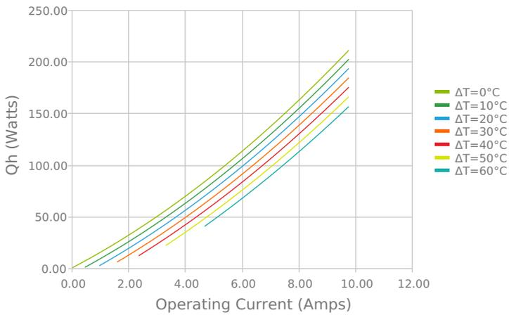
Total Heat Dissipated at Hot Side (Qh=Qc+Pin)
