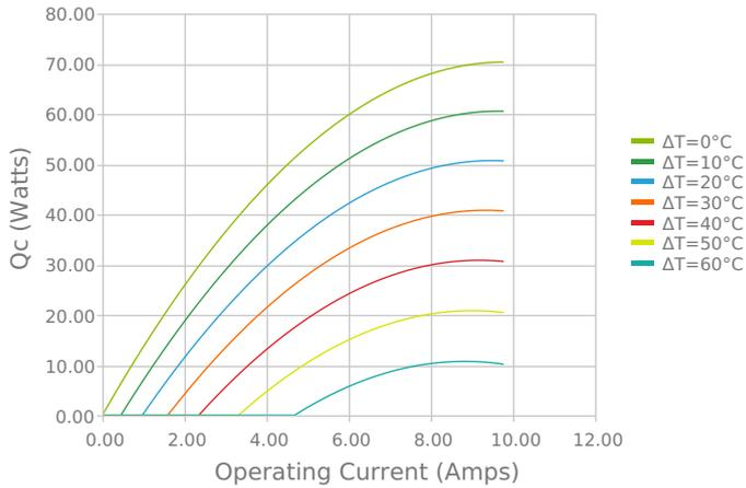
Heat Pumped at Cold Side
