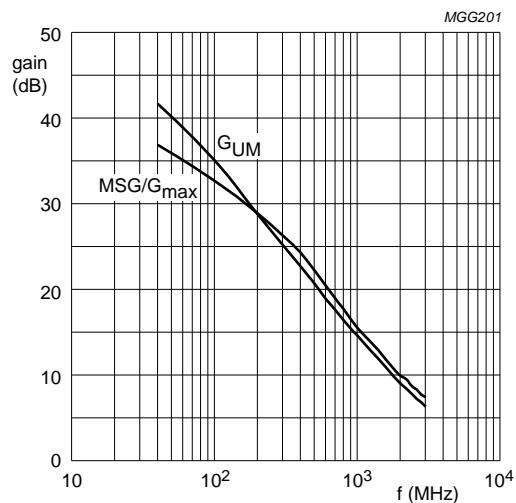
$I_C = 1 \text{ mA}; V_{CE} = 3 \text{ V.}$
