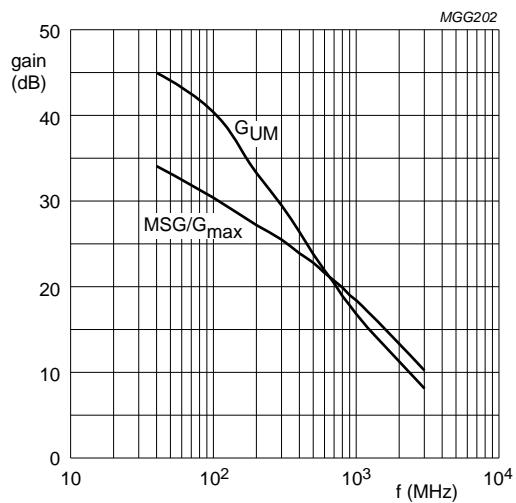
$I_C = 5 \text{ mA}; V_{CE} = 3 \text{ V.}$
