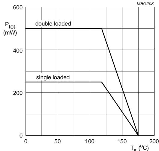
Fig.2 Power derating as a function of soldering point temperature; typical values.
