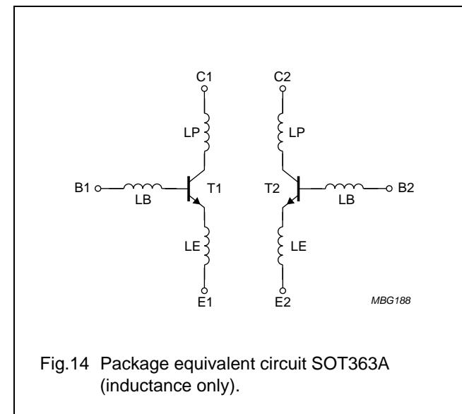
Fig.14 Package equivalent circuit SOT363A (inductance only).
