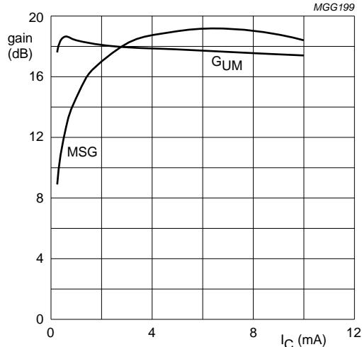
$f = 900 \text{ MHz}; V_{CE} = 3 \text{ V.}$
