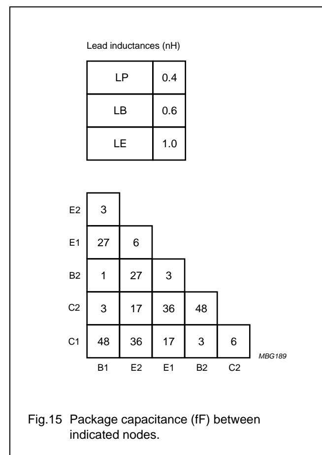
Fig.15 Package capacitance (fF) between indicated nodes.
