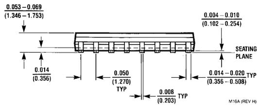
**16-Lead Small Outline Integrated Circuit (SOIC), JEDEC MS-012, 0.150" Narrow
