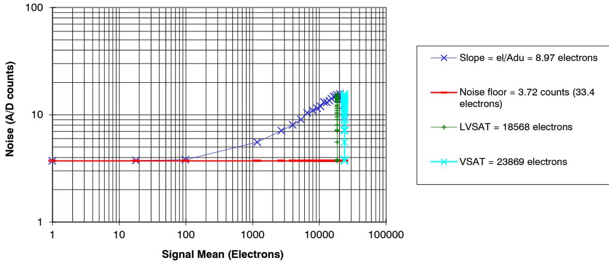
Figure 2. Measured Performance – Dynamic Range and Noise Floor
