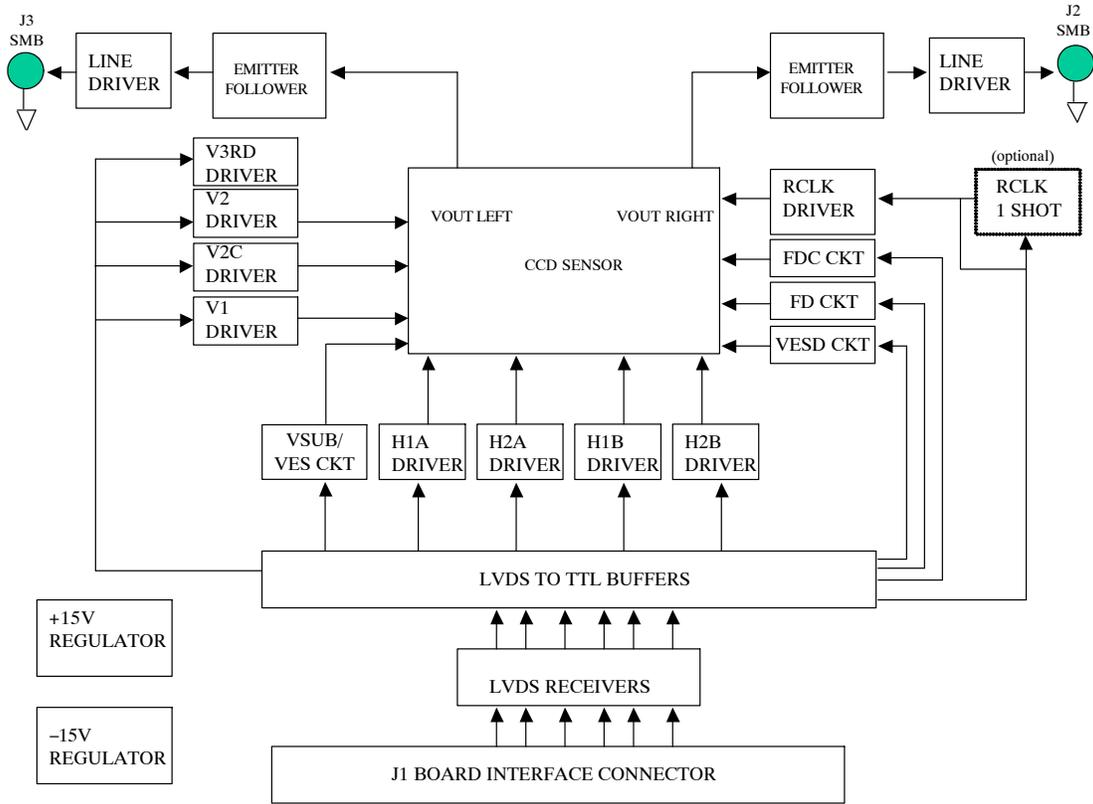
Figure 1. KAI-0340 Imager Board Block Diagram
