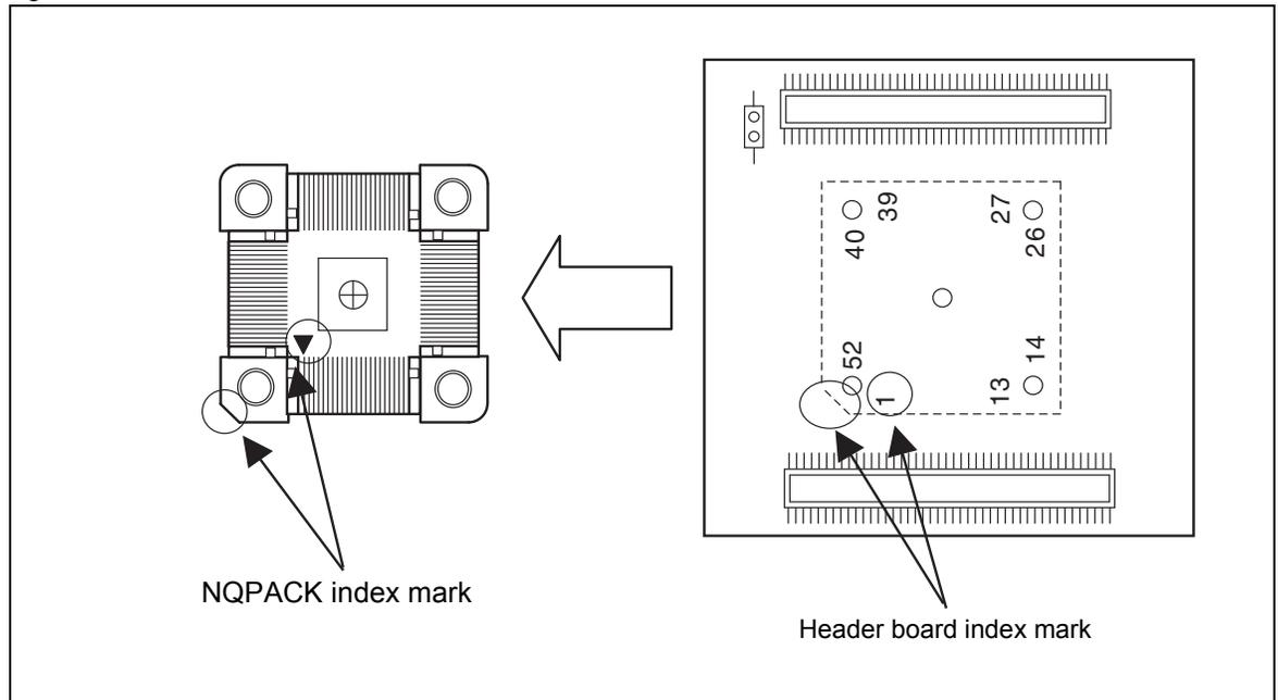
2. Insert each screw for securing the header board into each of the four tapped holes on the header board, and then tighten the screws diagonally. The center screw hole is not used. To tighten the screws, use the special screwdriver supplied with the NQPACK to equally tighten the four screws in sequence. Tightening the screws too tight might result in a defective contact.
