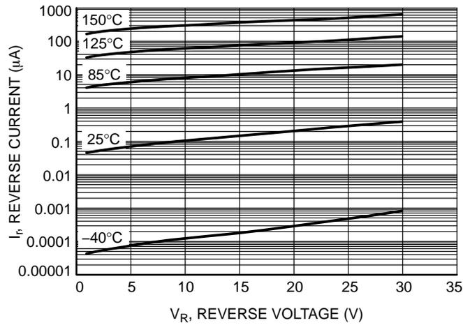
**Figure 3. Leakage Current**
