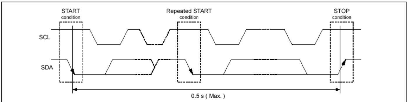
Fig.5 Starting and stopping on I<sup>2</sup>C bus
