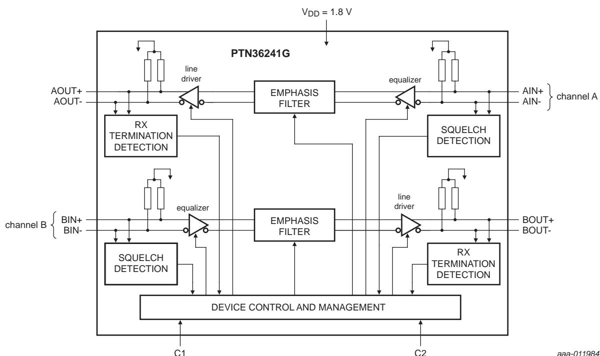
**Fig 2. Block diagram of PTN36241G**
