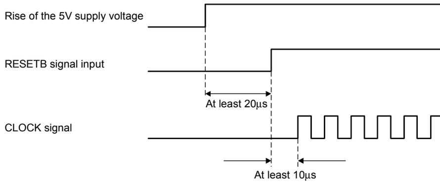
Figure 2 RESETB and CLOCK Signals Input Timing
