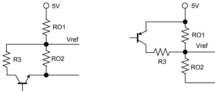
**Input Pin Functions (CMOS input levels)**
