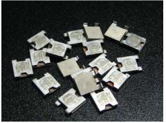
The Zener diode used for voltage clamping in a PolyZen microassembly was selected due to its relatively flat voltage vs current response. This helps improve output voltage clamping, even when input voltage is high and diode currents are large.
