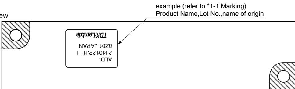
When LED driver is fixing, please confirm screw head and plate form is located within above hatching area include any tolerances. Please insulate it with the case such as sheet metals. Tolerance is  $\pm 0.5\text{mm}$  unless otherwise specified.
