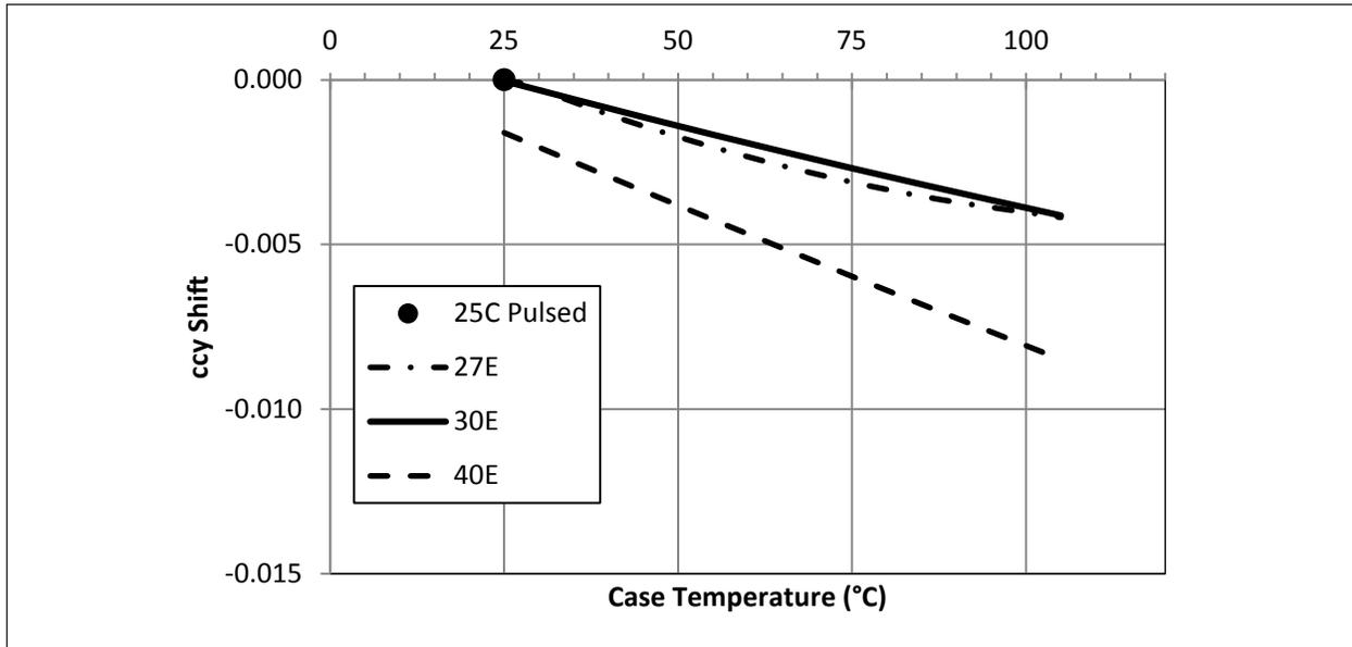
**Figure 6: Typical DC ccx Shift vs. Case Temperature**
