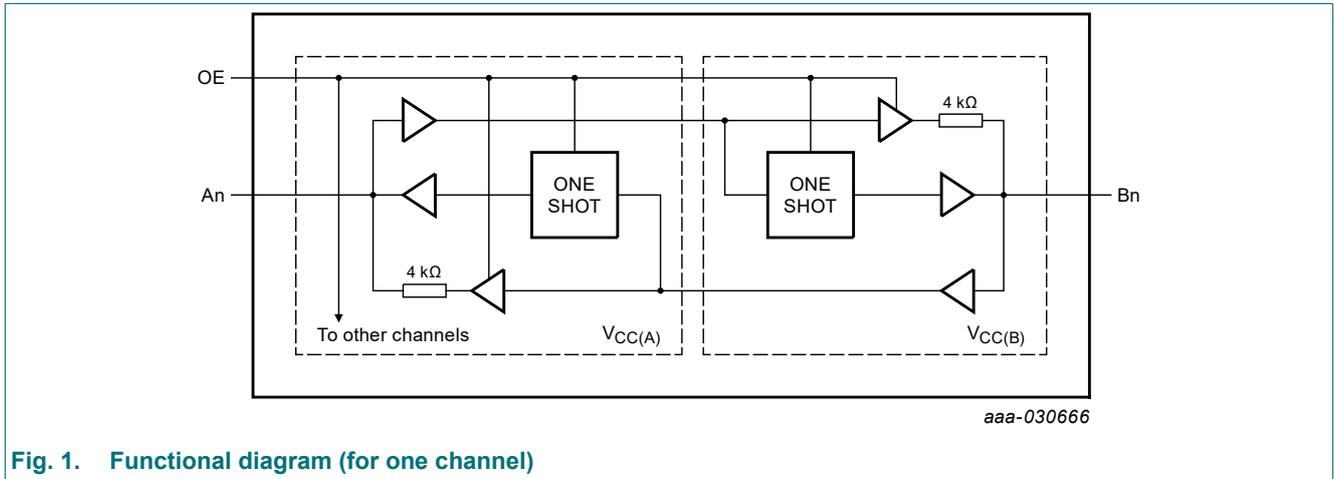
Fig. 1. Functional diagram (for one channel)
