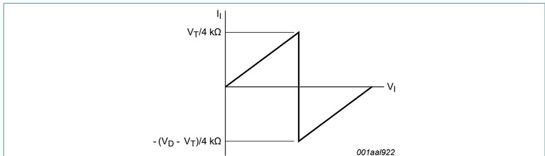
$V_T$ : input threshold voltage of the NXB0108 (typically  $V_{CC1} / 2$ ).
