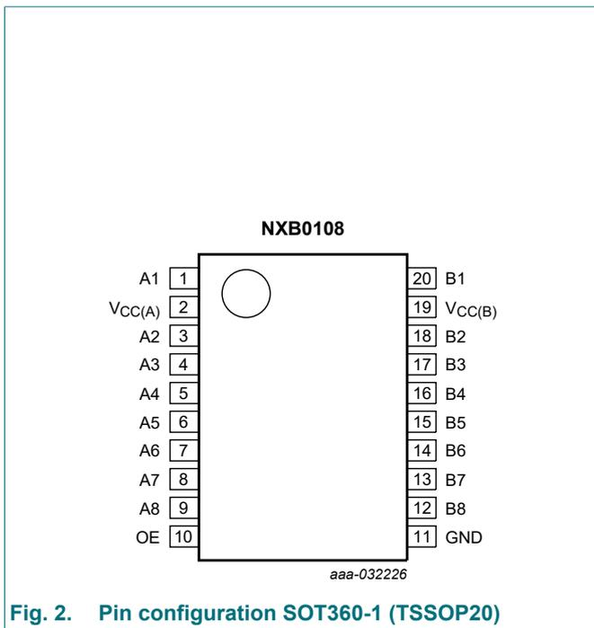
Fig. 2. Pin configuration SOT360-1 (TSSOP20)
