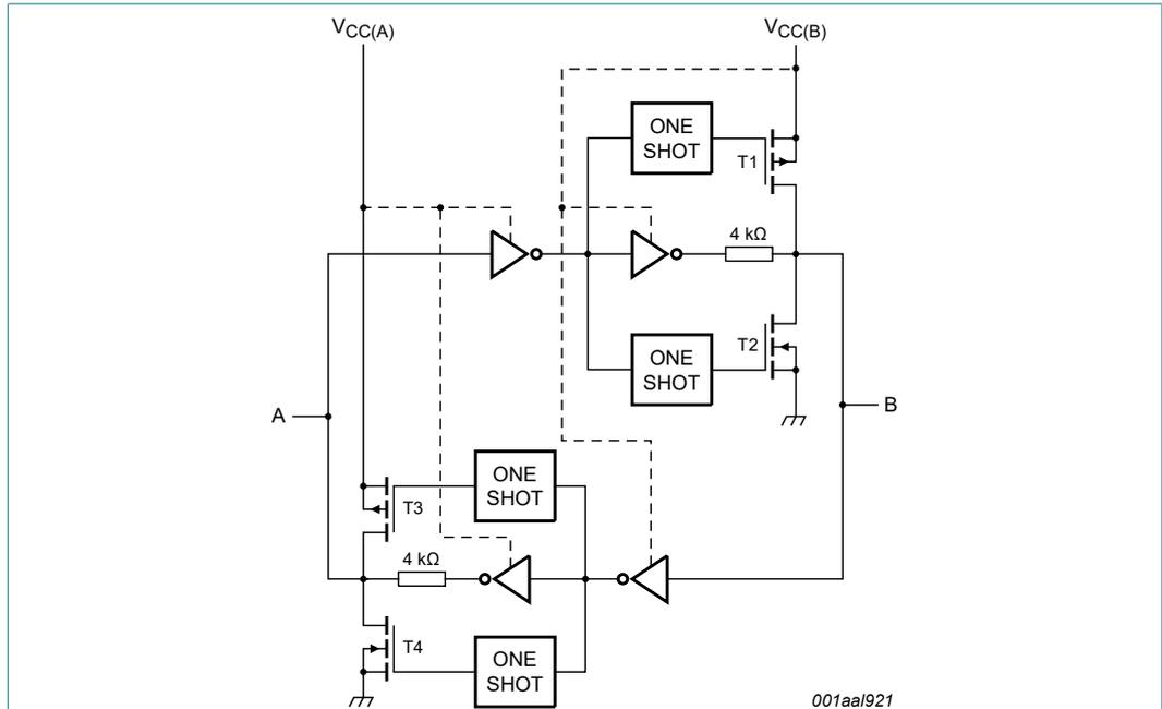
Fig. 8. Architecture of NXB0108 I/O cell (one channel)
