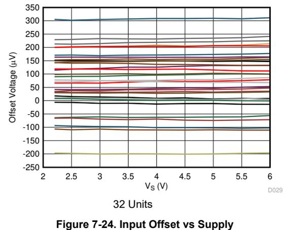
Figure 7-24. Input Offset vs Supply
