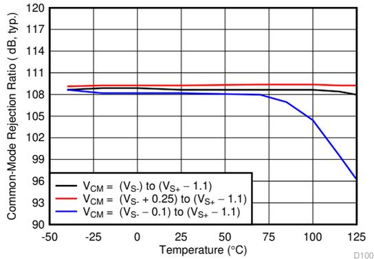
Figure 7-25. Common Mode Rejection Ratio vs Temperature
