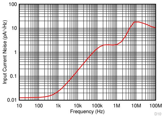
Figure 7-3. Input Current Noise Density vs Frequency
