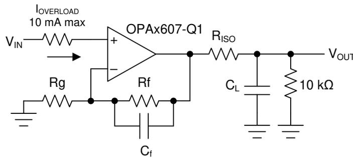
**Figure 8-1. Input Current Protection and Driving Capacitive Loads**
