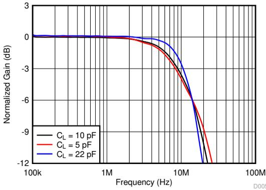
Figure 7-5. Small-Signal Frequency Response vs Capacitive Load
