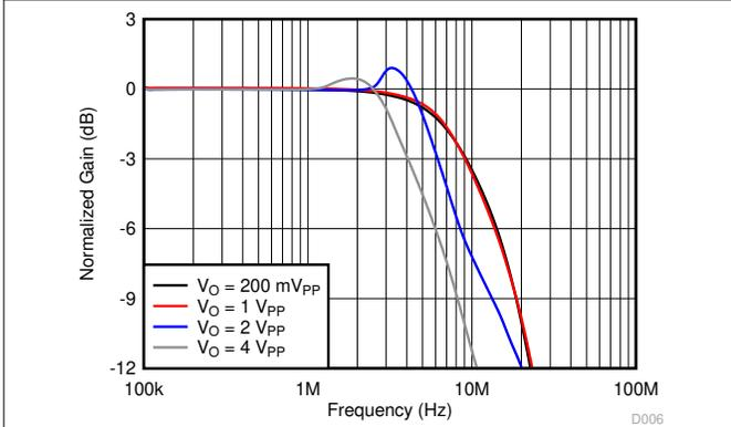
**Figure 7-7. Large-Signal Frequency Response vs Output Voltage**
