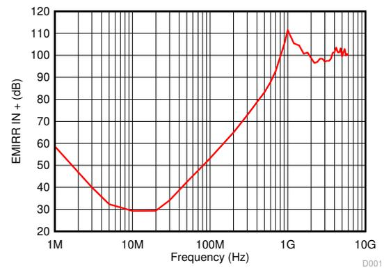
Figure 7-30. Electromagnetic Interference Rejection Ratio Referred to Noninverting Input (EMIRR+) vs Frequency
