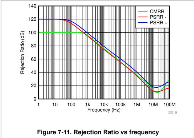
**Figure 7-11. Rejection Ratio vs frequency**
