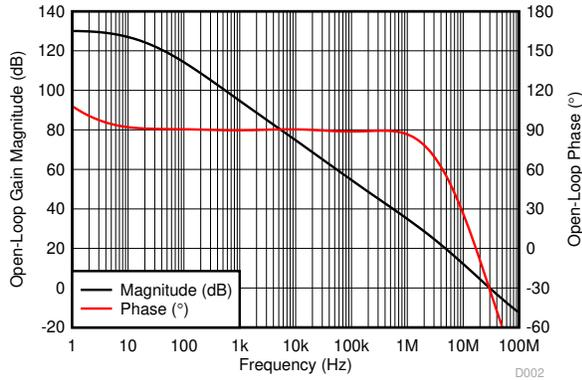
Figure 7-1. Open Loop Gain and Phase vs Frequency
