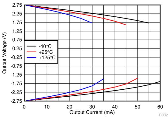
Figure 7-29. Output Voltage vs Output Current Sourcing and Sinking
