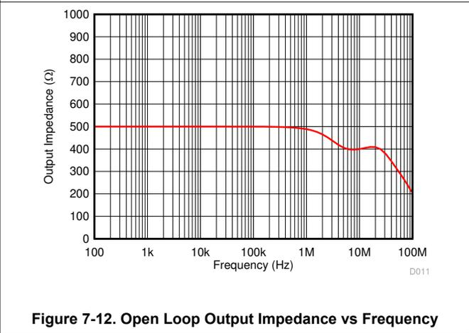
**Figure 7-12. Open Loop Output Impedance vs Frequency**
