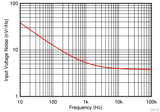
Figure 7-2. Input Voltage Noise Density vs Frequency
