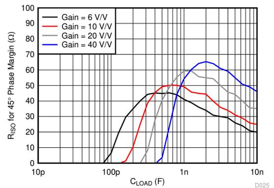
**Figure 7-18. Recommended Isolation Resistor vs Capacitive Load**
