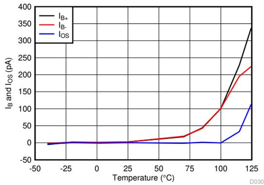
Figure 7-27. Input Bias and Offset Current vs Temperature
