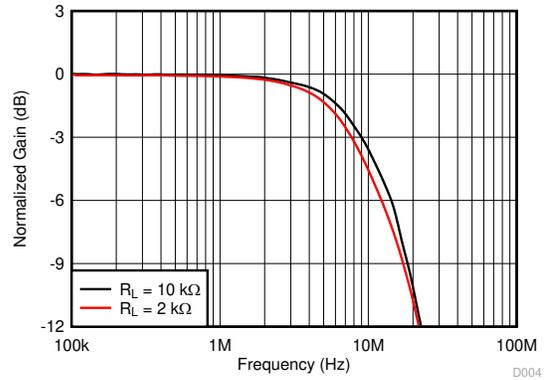
Figure 7-6. Small-Signal Frequency Response vs Output Load
