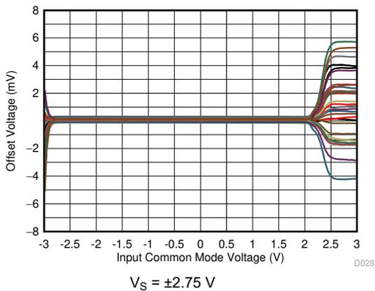
Figure 7-23. Input Offset vs Common Mode Voltage
