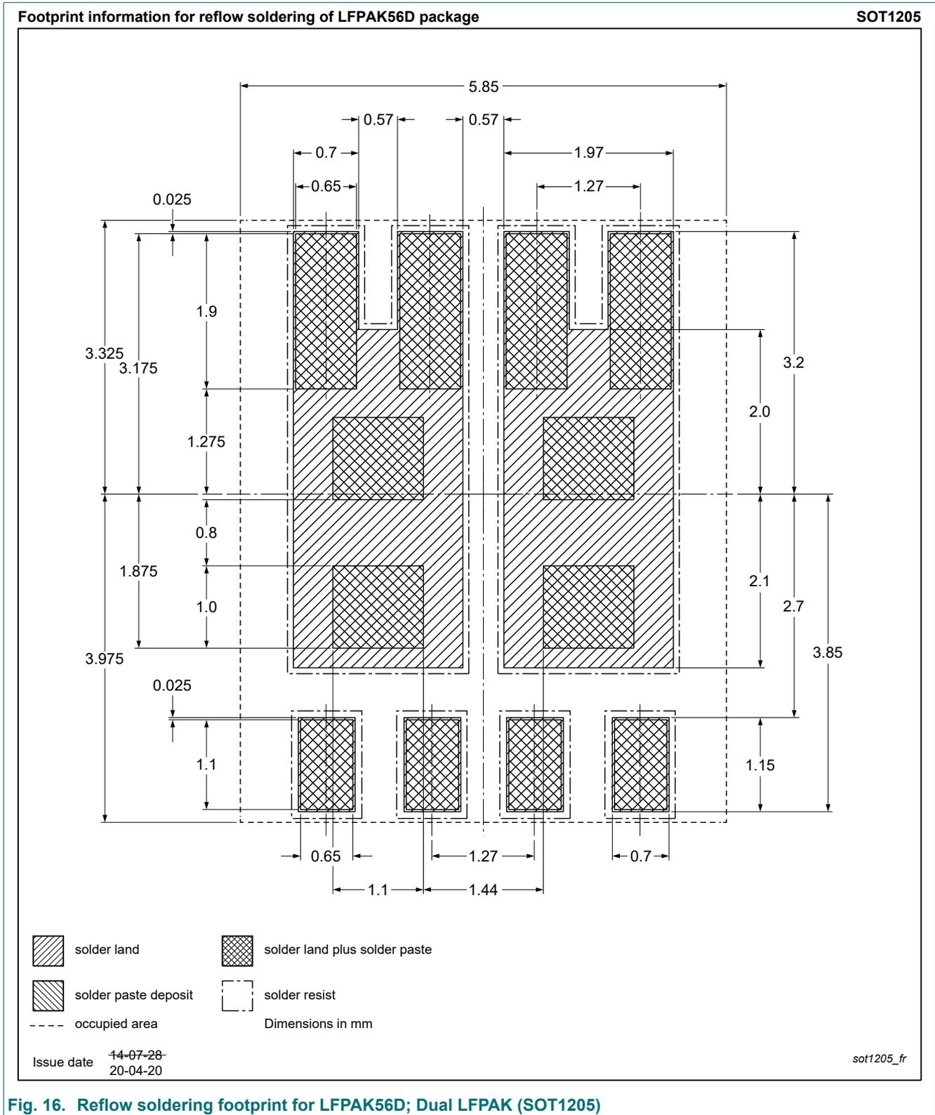
Fig. 16. Reflow soldering footprint for LPAK56D; Dual LPAK (SOT1205)
