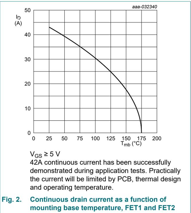
Dual N-channel 40 V, 13 mOhm standard level MOSFET in LPAK56D (half-bridge configuration)
