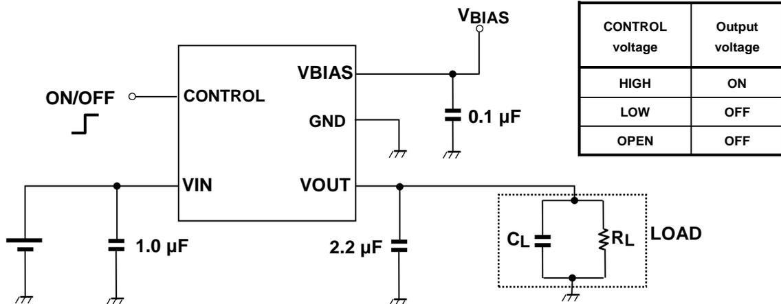
The figure above shows the Example of configuration for using a Low dropout regulator. Insert a capacitor at VIN, VOUT and VBIAS pins for stable input/output operation. (Ceramic capacitors can be used).
