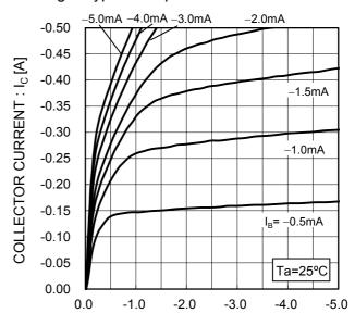
COLECTOR TO EMITTE VOLTAGE: V<sub>CE</sub>[V]
