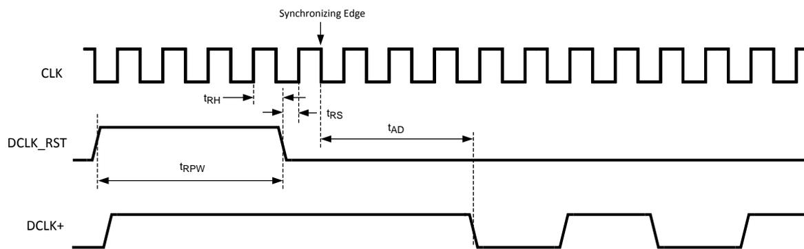
Figure 6. Clock Reset Timing in DDR Mode
