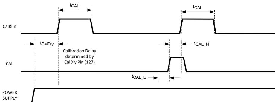
**Figure 9. Self Calibration and On-Command Calibration Timing**
