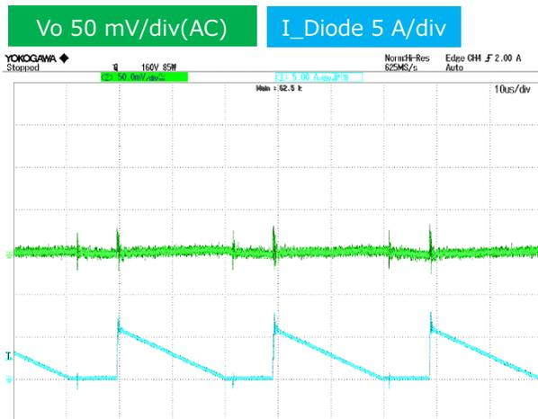
Figure 28. Output Ripple Voltage  $V_{in\_dc} = 300\text{ V}$ ,
