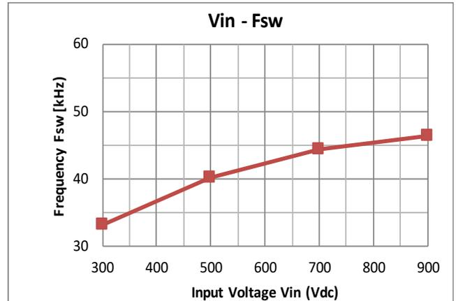
Figure 9. Input Voltage  $V_{in}$  vs Frequency ( $I_o = 2$  A)
