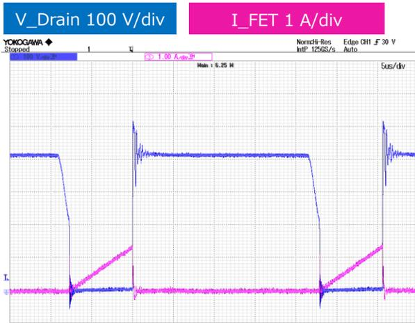
Figure 14.  $V_{in\_dc} = 300\text{ V}$ ,  $I_o = 2.0\text{ A}$
