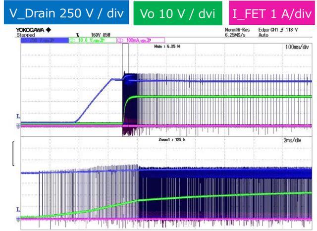
Figure 23. Startup  $V_{in\_dc} = 900\text{ V}$ ,  $I_o = 0\text{ A}$
