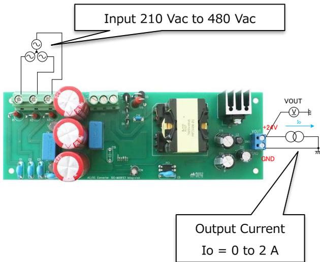
Figure 2. Input with 3-phase AC power supply
