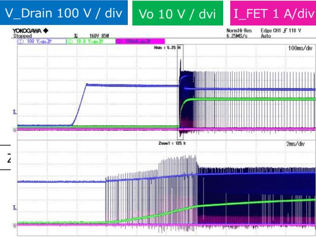
Figure 22. Startup  $V_{in\_dc} = 300\text{ V}$ ,  $I_o = 0\text{ A}$
