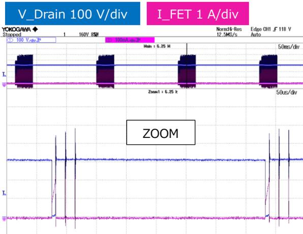
Figure 18. Output short  $V_{in\_dc} = 300\text{ V}$
