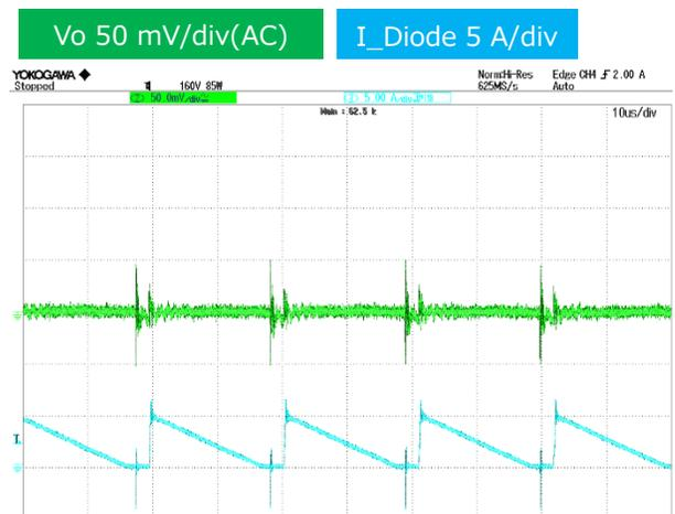
Figure 29. Output Ripple Voltage  $V_{in\_dc} = 900\text{ V}$ ,
