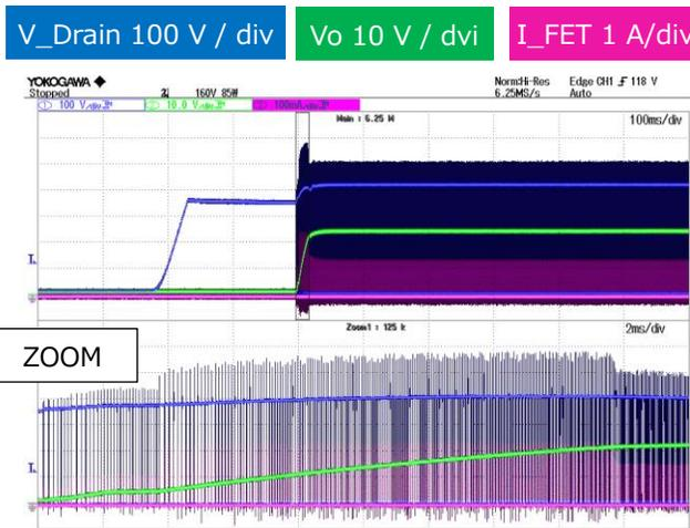
Figure 24. Startup  $V_{in\_dc} = 300\text{ V}$ ,  $I_o = 2\text{ A}$
