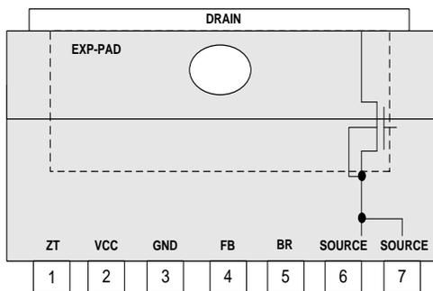
Figure 4. Pin Configuration
