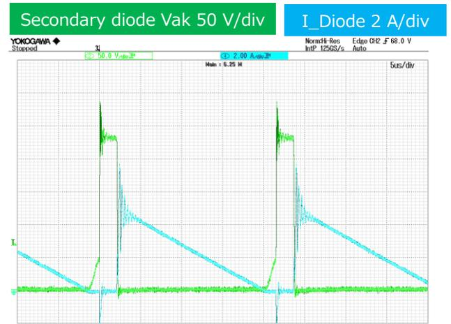
Figure 17.  $V_{in\_dc} = 900\text{ V}$ ,  $I_o = 2.0\text{ A}$
