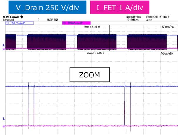
Figure 19. Output short  $V_{in\_dc} = 900\text{ V}$
