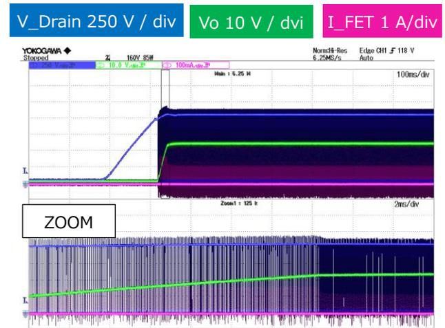
Figure 25. Startup  $V_{in\_dc} = 900\text{ V}$ ,  $I_o = 2\text{ A}$
