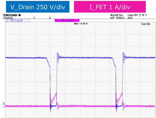
Figure 15.  $V_{in\_dc} = 900\text{ V}$ ,  $I_o = 2.0\text{ A}$
