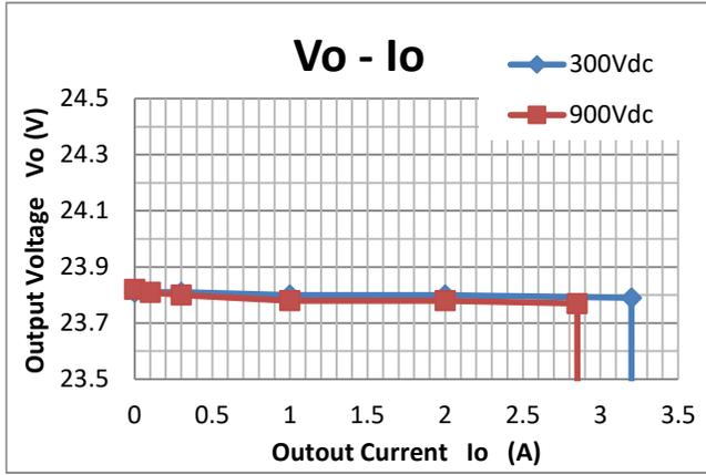
Figure 6. Output Voltage vs Output Current –
