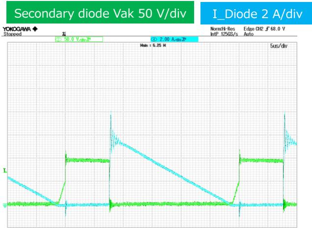
Figure 16.  $V_{in\_dc} = 300\text{ V}$ ,  $I_o = 2.0\text{ A}$
