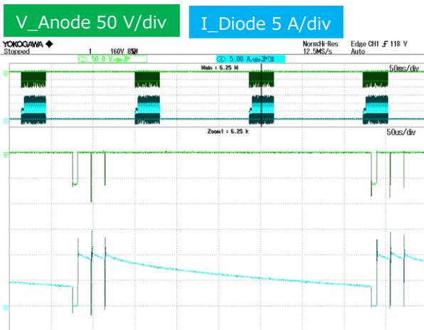
Figure 20. Output short  $V_{in\_dc} = 300\text{ V}$
