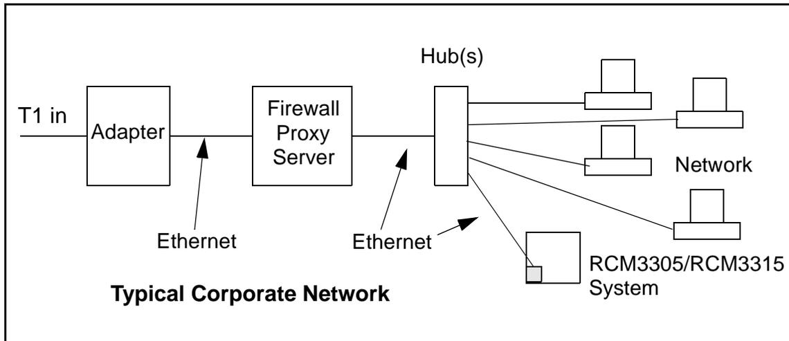
If your system administrator can give you an Ethernet cable along with its IP address, the netmask and the gateway address, then you may be able to run the sample programs without having to setup a direct connection between your computer and the RCM3305/RCM3315. You will also need the IP address of the nameserver, the name or IP address of your mail server, and your domain name for some of the sample programs.
