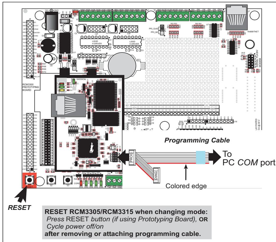
**Figure 8. Switching Between Program Mode and Run Mode**
