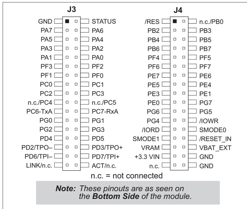
**Figure 5. RCM3305/RCM3315 Pinouts**
