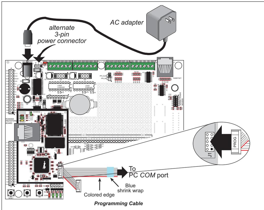
**Figure 3(b). Connect Programming Cable and Power Supply**
