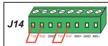
Once you have compiled and run this program, you can test flow control by disconnecting TxF from RxF while the program is running. Characters will no longer appear in the **STDIO** window, and will display again once TxF is connected back to RxF.
