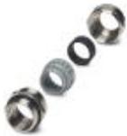
Metal screw connection up to 5 bar, thread length: 8 mm, cable diameter: 19 - 27 mm, WAF 43, screw connection: M32
