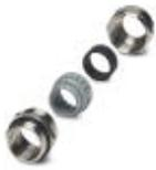
Metal screw connection up to 5 bar, thread length: 8 mm, cable diameter: 14 - 21 mm, WAF 34, screw connection: M32
