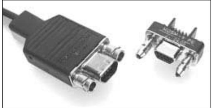
The push/pull latching system is designed for applications which require a quick connect and disconnect. A spring retention mechanism latches to a post on the board side to prevent unintentional unmatings.
