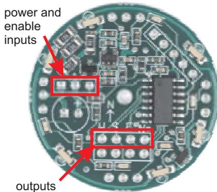
There are two sets of electrical connections to the IR beacon. Three pins on the "west" side are for power and an optional enable input. Apply 6-16 V across the + and - pins; making the enable pin high (5 V) will enable the beacon (both transmission and reception). The four directional outputs are located on the "south" side of the PCB. Each pin is normally high (5 V), and it will go low (0 V) if the other beacon is detected in the corresponding direction.
