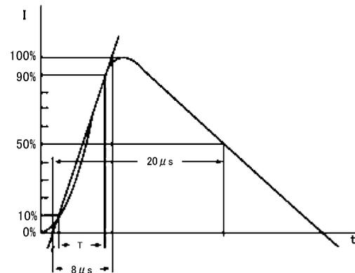
Fig. 6.3.2 Based on IEC61000-4-5 8/20  $\mu\text{s}$  pulse.
