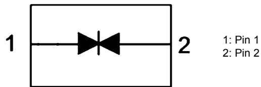
Note: Connect Pin 2 to GND when using Pin 1 for I/O.
