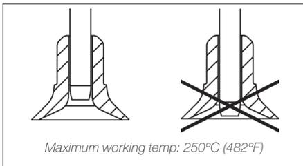
Insert the needle with the appropriate cup for a correct suction process.
