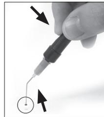
Once the suction is activated, cover the pen hole with your finger and lift off the component.
