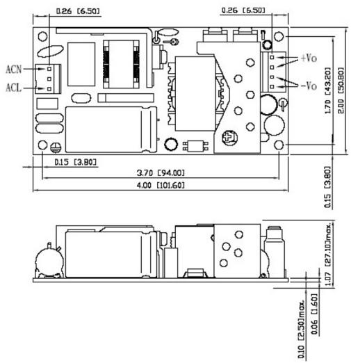
Four mounting holes 0.13" [3.3mm] in diameter
