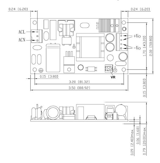
Four mounting holes 0.13" [3.3mm] in diameter
