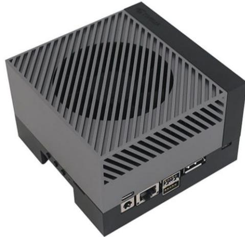
NVIDIA® Jetson AGX Orin™ Developer Kit, provides a giant leap forward for Robotics and Edge AI. With up to 275 TOPS of AI performance and power configurable between 15W and 50W, you now have more than 6X the performance of NVIDIA® Jetson AGX Xavier™ in the same compact form-factor for developing advanced robots and other autonomous machine products.
