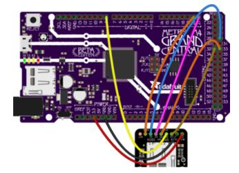
Board 3.3 to breakout 3V Board GND to breakout GND Board D32 to breakout CLK Board D33 to breakout CMD Board D8 to breakout D0 Board D29 to breakout D1 Board D20 to breakout DAT2 Board D21 to breakout D3 To mount the SD card, use the following code. Remember to put it in the file mount\_s d.py on CIRCUITPY so you can easily call it from code.py or the REPL with import mount\_sd.
