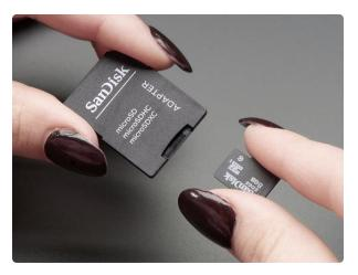
SD/MicroSD Memory Card (8 GB SDHC) Add mega-storage in a jiffy using this 8 GB class 4 micro-SD card. It comes with a SD adapter so you can use it with any of our shields or adapters. Preformatted to FAT so it works out...
