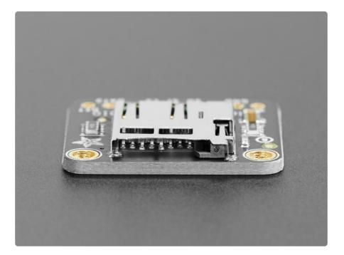
You will need to verify that your microcontroller has SDIO support and you have SDIO firmware/library support as well. SDIO is usually available on higher end chips, and you may need to use some specific pins. You can still use this for SPI mode, but it does not have level shifters, so it's not for use with 5V microcontrollers.
