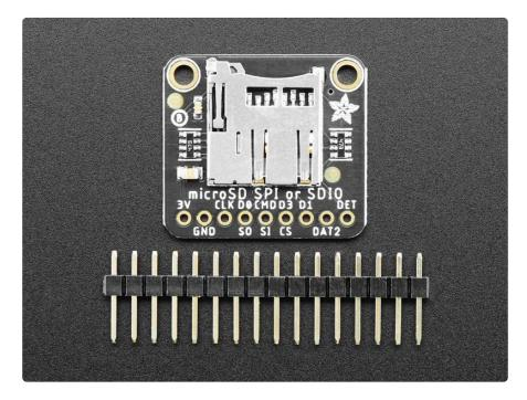
With the Adafruit MicroSD SPI or SDIO Card Breakout Board, you can add an SD card to your project using the common SPI interface or the higher performance SDIO interface.
