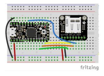
Board 3V to breakout 3V via supply rail Board GND to breakout GND via supply rail
