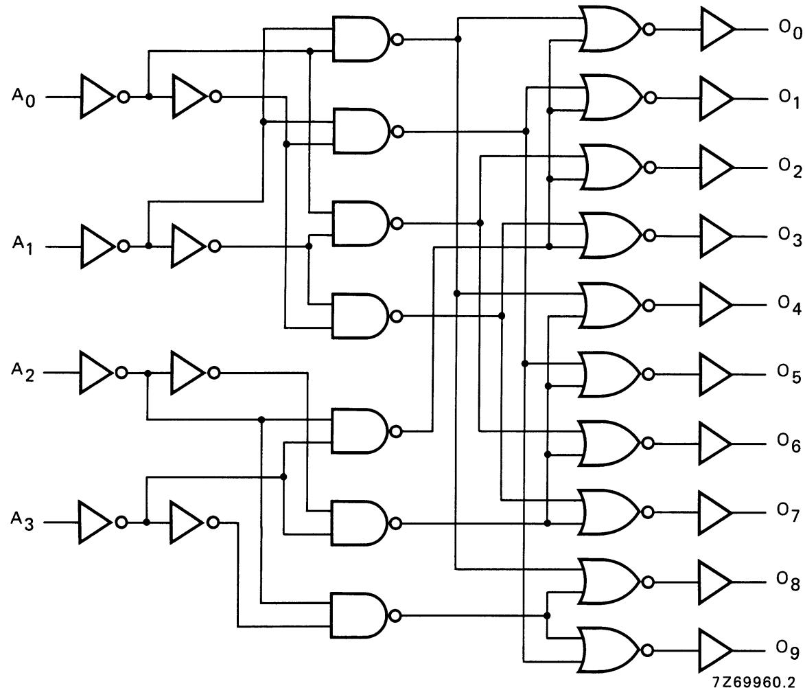
Fig.3 Logic diagram.
