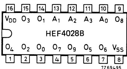
Fig.2 Pinning diagram.
