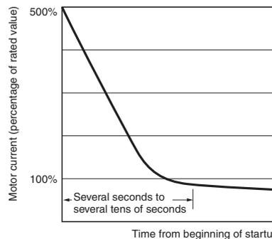
For a motor with a rating of 5 A, the startup current will be approximately 30 A. The startup current will exceed the overload capacity (rating: 150% for 1 s) of the K8AK-AW1 and K8AK-AW2 and result in failure of the Relay. To monitor the motor load, use the K8AK-AW3. (Overload capacity: 120% of rating for continuous load, 200% of rating for 30 s, and 600% of rating for 1 s). The K8AK-AW3 has a large input range. Pass the conductors multiple times through the special CT.
