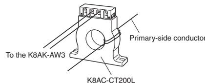
**Concept behind Passing Conductor through the CT When Using the K8AK-AW3**
