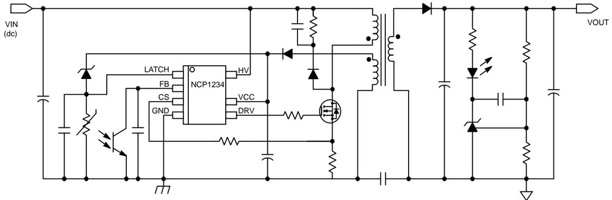
Figure 1. Flyback Converter Application Using the NCP1234
