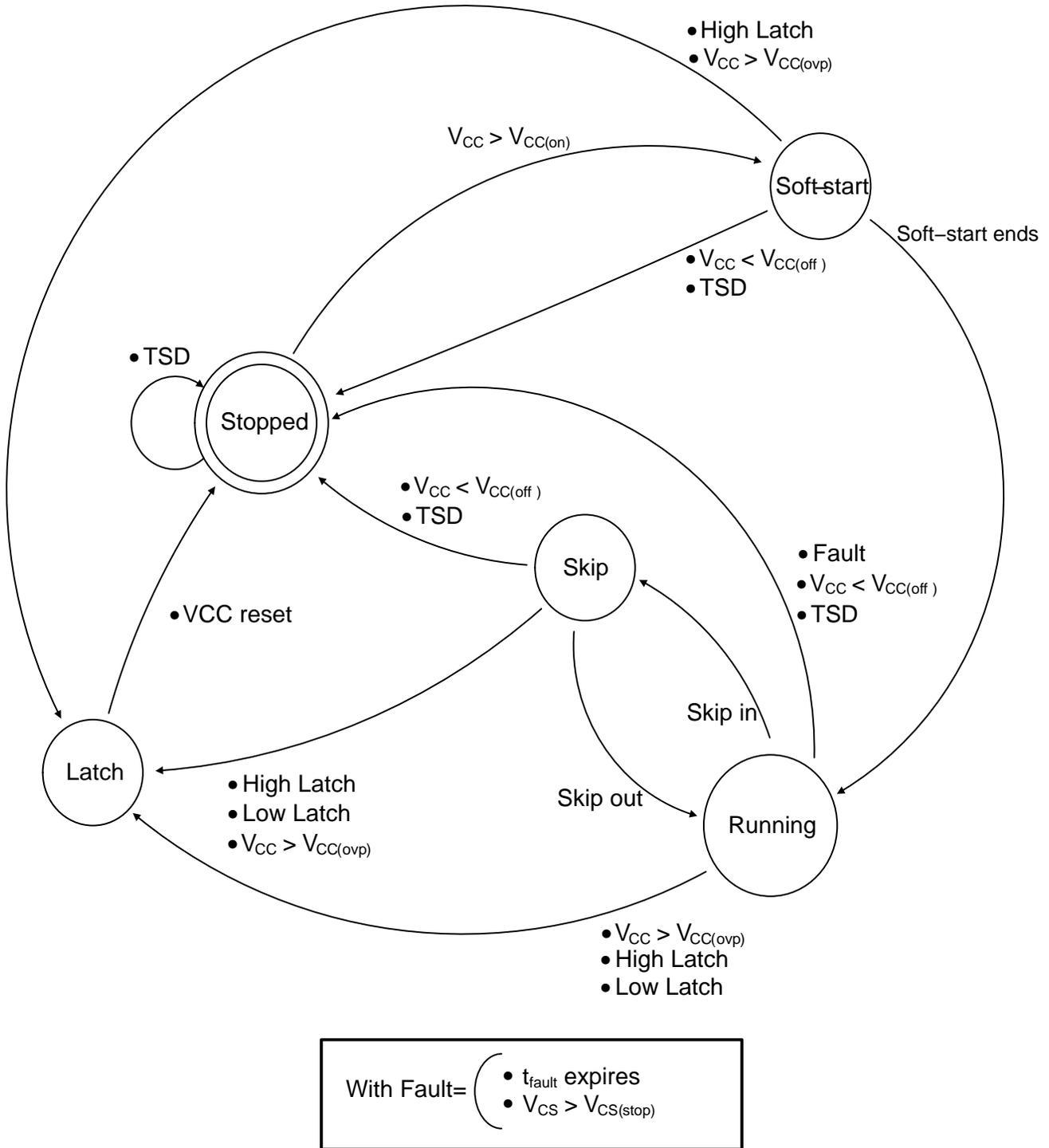
Figure 49. Controller Operation State Diagram (Latched Protection)
