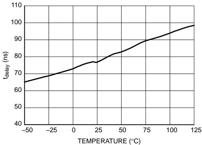
Figure 7. Propagation Delay t<sub>delay</sub>
