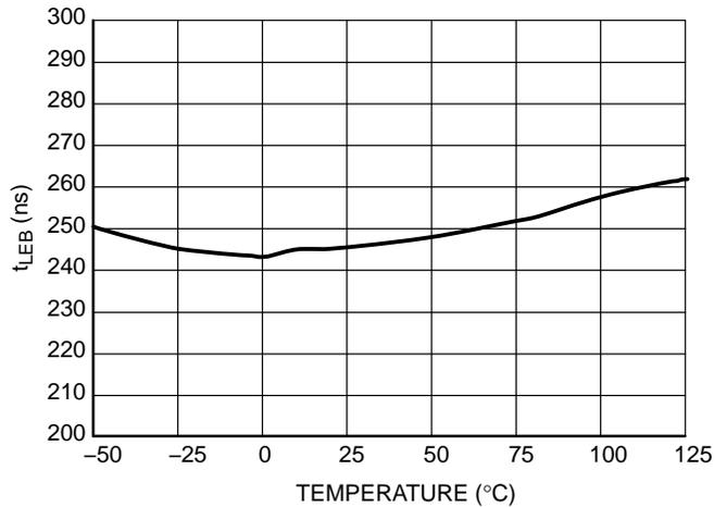
Figure 8. Leading Edge Blanking Duration t<sub>LEB</sub>
