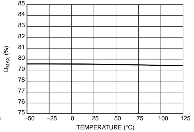
Figure 12. Maximum Duty Cycle  $D_{MAX}$
