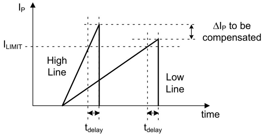
Figure 34. Line Compensation for True Overpower Protection
