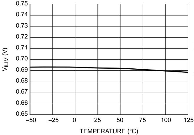
Figure 5. Maximum Internal Current Setpoint
