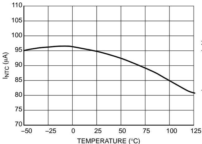
Figure 25. Current I<sub>NTC</sub> Sourced from the Latch Pin, Allowing Direct NTC Connection
