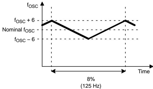
**Figure 30. Frequency Jittering**
