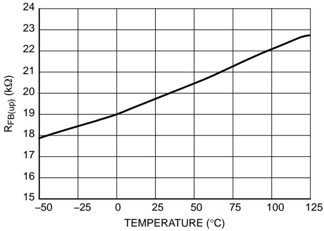
Figure 9. FB Pin Internal Pull-up Resistor  $R_{FB(up)}$
