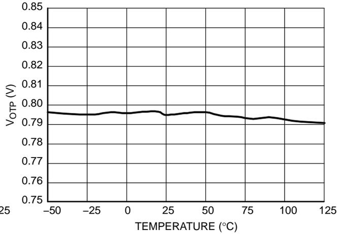
Figure 22. Latch Pin Low Threshold V<sub>OTP</sub>
