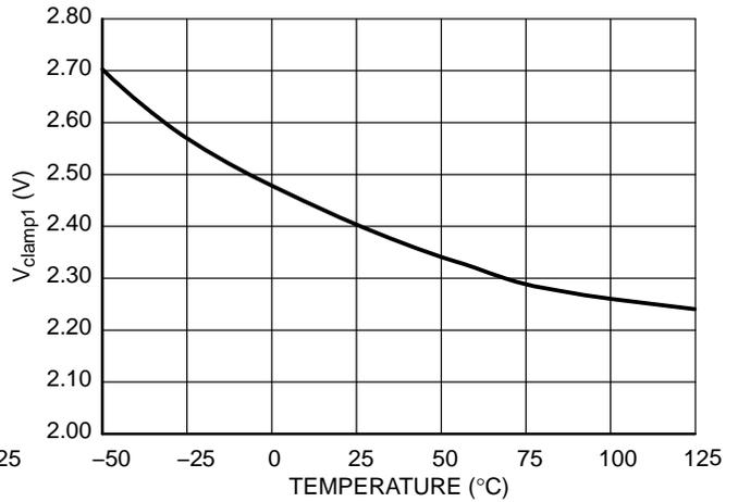
Figure 24. Latch Pin Voltage V<sub>clamp1</sub> (Latch-off Pin is Sinking 1 mA)
