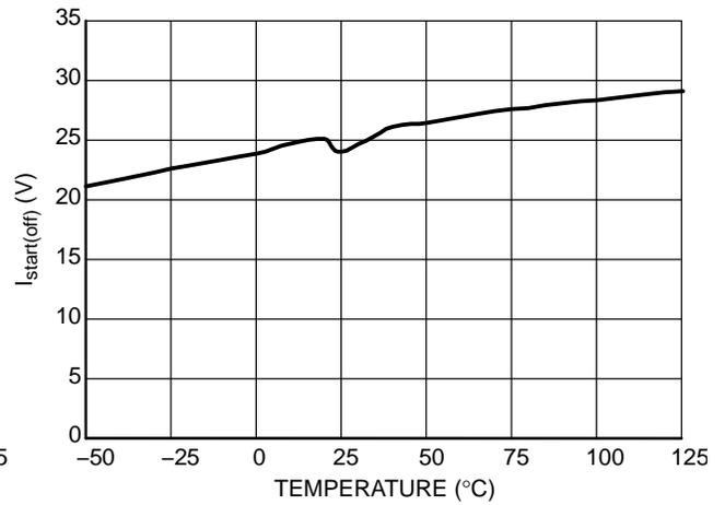
Figure 4. Off-State Leakage Current I<sub>start(off)</sub>
