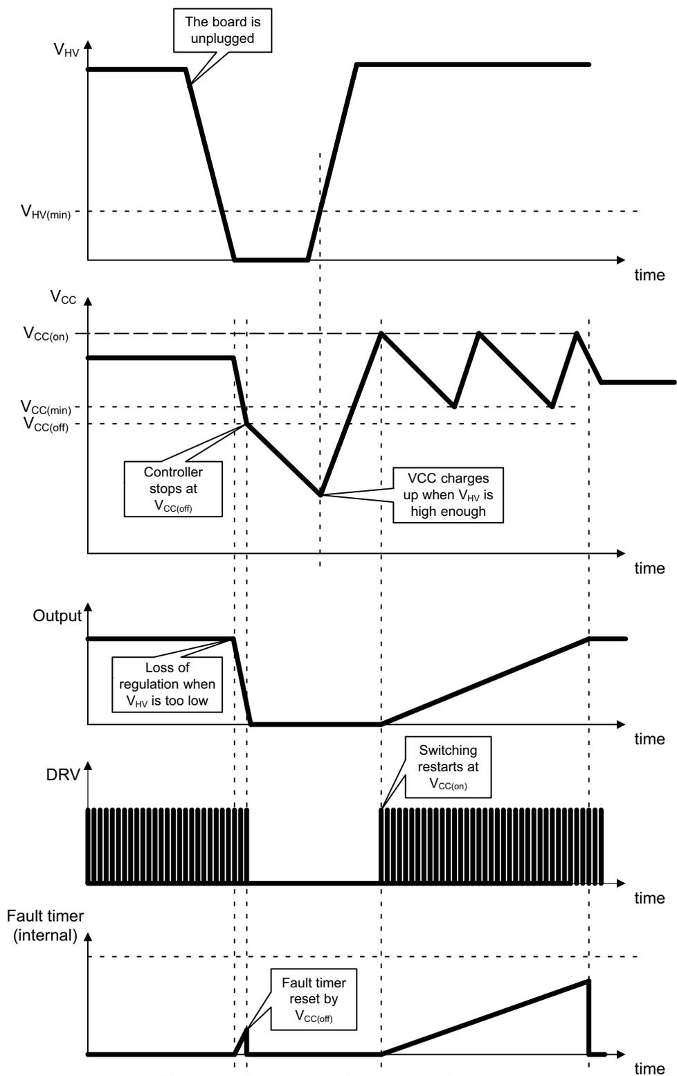
Figure 29. Fast Application Off – On Sequence
