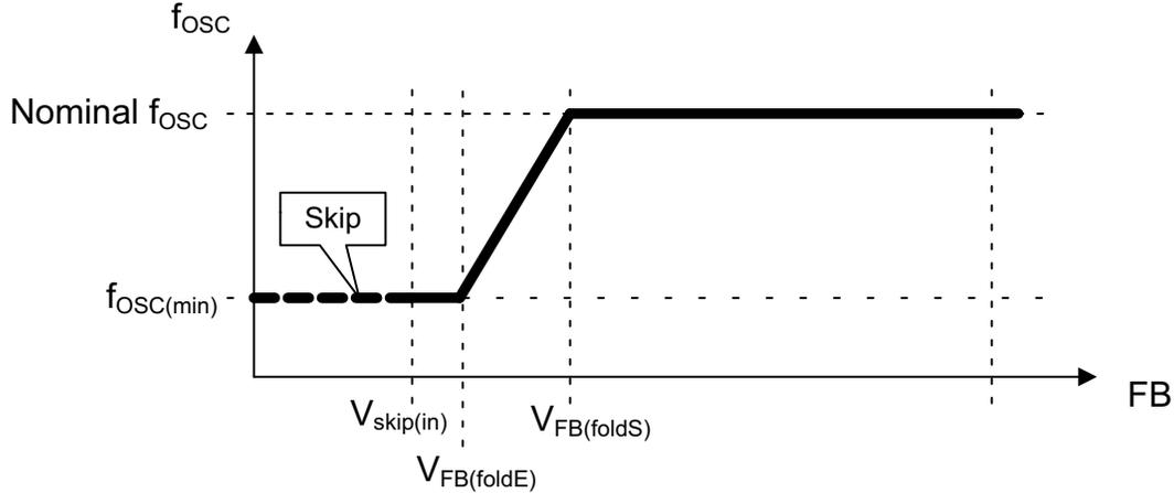
Figure 43. Frequency Foldback when the FB Voltage Decreases
