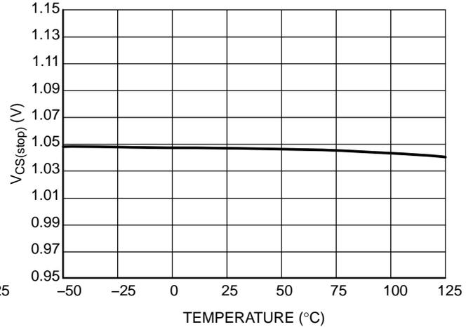
Figure 6. Threshold for Immediate Fault Protection Activation V<sub>CS(stop)</sub>
