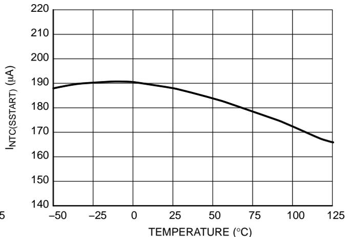
Figure 26. Current I<sub>NTC(SSSTART)</sub> Sourced from the Latch Pin, During Soft-Start
