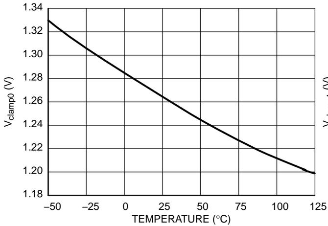
Figure 23. Latch Pin Open Voltage V<sub>clamp0</sub>
