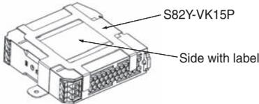
Side mounting is only for S8VK-G015□□. Use a mounting bracket (S82Y-VK15P, sold separately) when the product is mounted horizontally. Heat dissipation will be adversely affected. When the product is mounted facing horizontally, always place the side with label facing upward.
