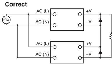
**Note: 1.** The diode is connected as shown in the figure. If the load is short-circuited, a reverse voltage will be generated inside the Power Supply. If this occurs the Power Supply may possibly deteriorate or be damaged. Always connect a diode as shown in the figure. Select a diode having the following ratings.
