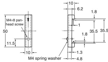
Note: If there is a possibility that the Unit will be subject to vibration or shock, use a steel DIN Rail. Otherwise, metallic filings may result from aluminum abrasion.
