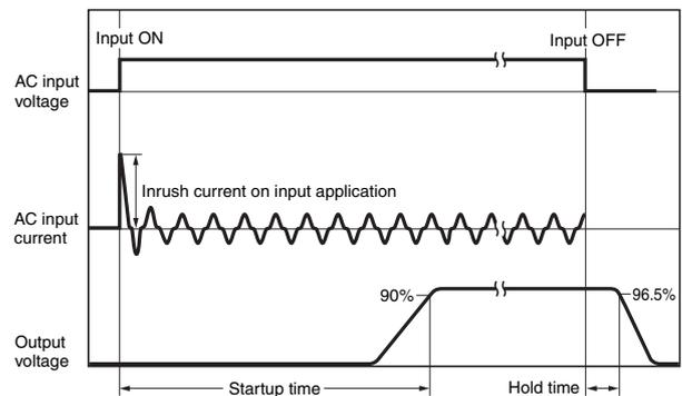
**Note:** Twice the input current or above will flow during the parallel operation or redundant system. Therefore, check the fusing characteristics of fuses and operating characteristics of breakers making sure that the external fuses will not burn out and the circuit breakers will not be activated by the inrush current.
