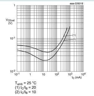
Collector-emitter saturation voltage as a Fig. 8. function of collector current; typical values
