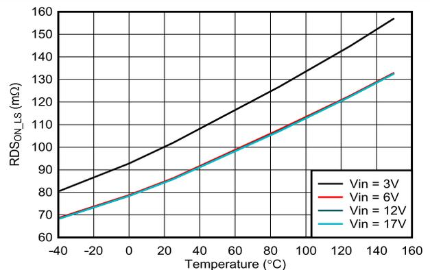
Figure 7-12. Low-Side RDS<sub>ON</sub> vs Temperature
