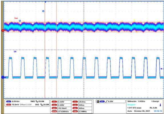
$V_{IN} = 12\text{ V}$        $L = 2.2\ \mu\text{H}$        $F_{SW} = 2.5\text{ MHz}$
