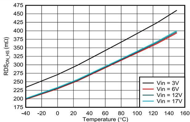
Figure 7-11. High-Side RDS<sub>ON</sub> vs Temperature
