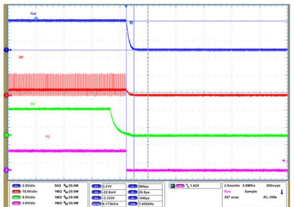
$V_{IN} = 12\text{ V}$        $L = 3.3\ \mu\text{H}$        $F_{SW} = 1.0\text{ MHz}$
