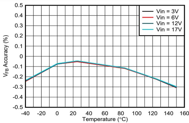
**Figure 7-3. Output Voltage Accuracy – External Feedback**
