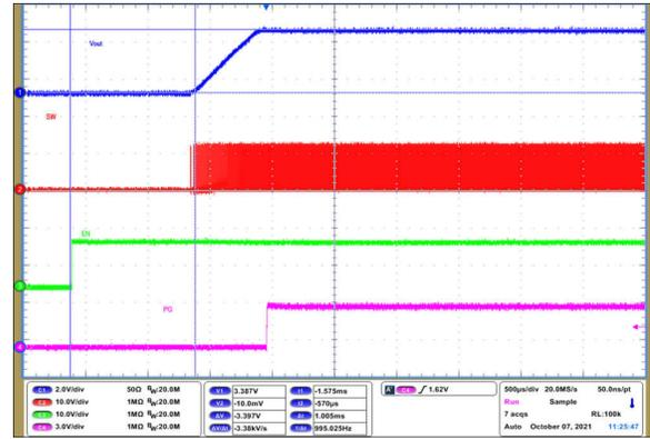
$V_{IN} = 12\text{ V}$        $L = 2.2\ \mu\text{H}$        $F_{SW} = 2.5\text{ MHz}$
