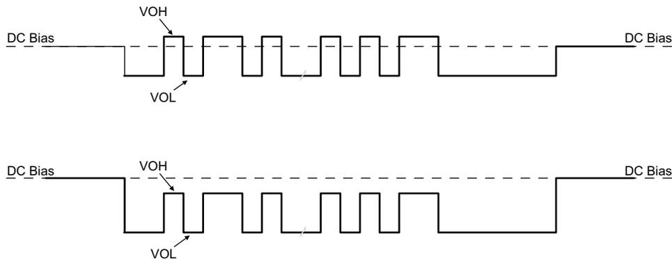
Figure 8-6. TX Driver Transmission with DC Bias
