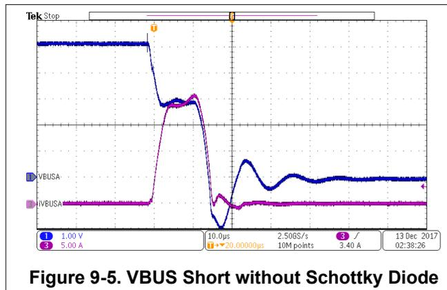
Figure 9-5. VBUS Short without Schottky Diode
