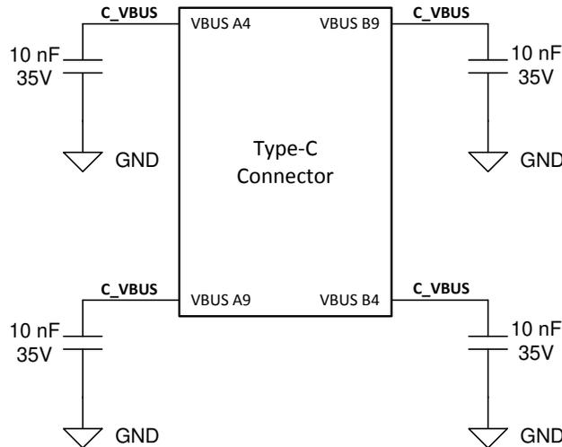
**Figure 9-3. Type-C Connector VBUS Capacitors**
