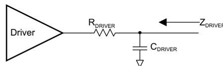
Figure 8-7.  $Z_{DRIVER}$  Circuit
