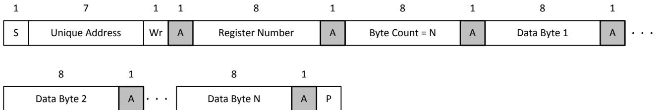
**Figure 8-26. I<sup>2</sup>C Unique Address Write Register Protocol**
