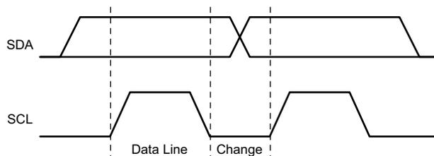
**Figure 8-24. I<sup>2</sup>C Bit Transfer**
