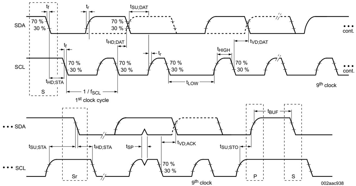
**Figure 7-1. I<sup>2</sup>C Slave Interface Timing**
