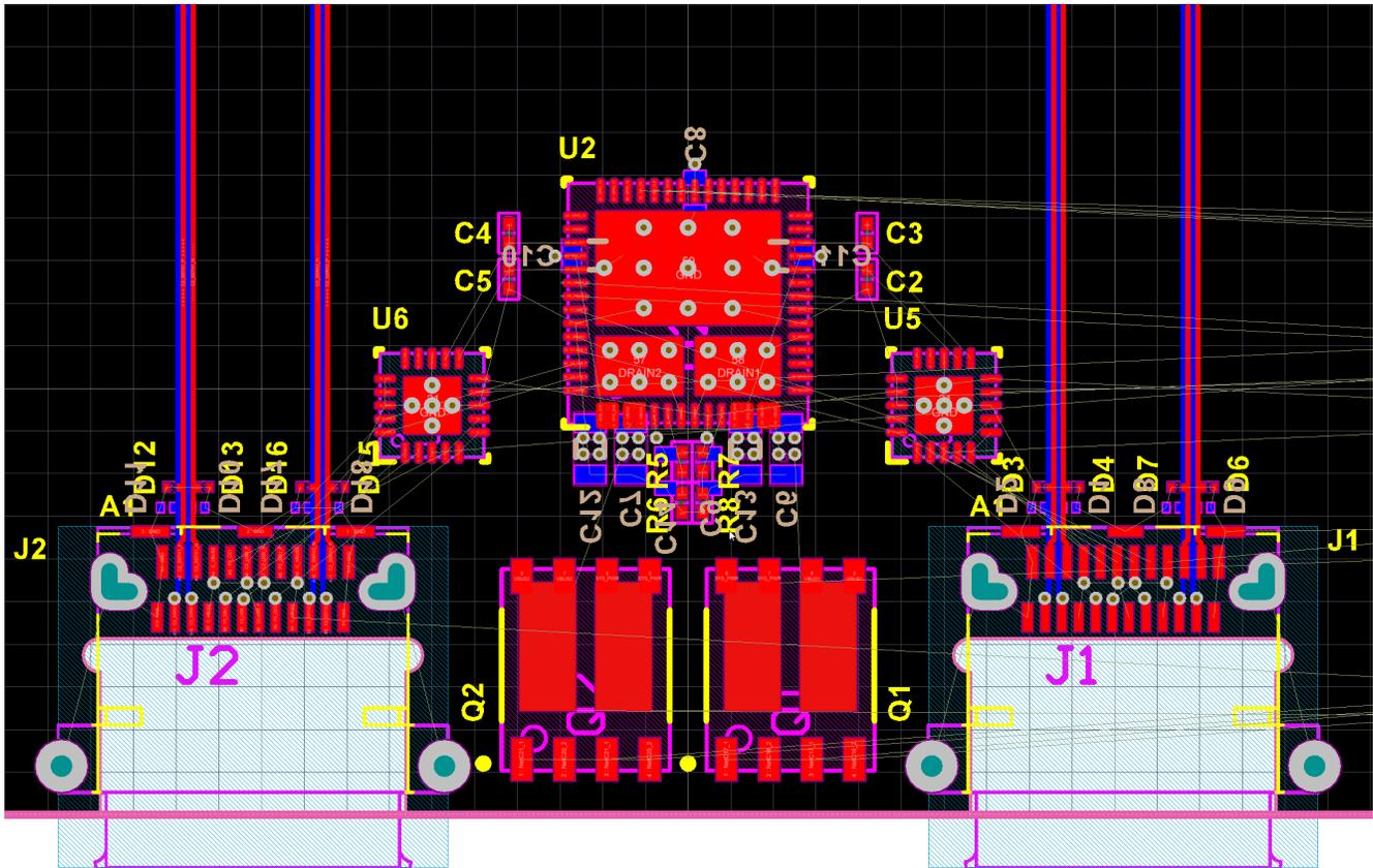
Figure 11-13. Protection Placement
