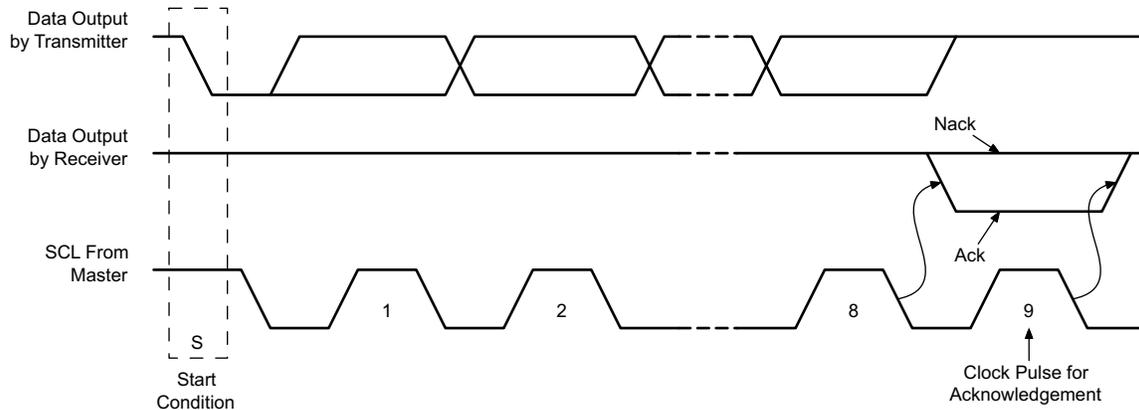
**Figure 8-25. I<sup>2</sup>C Acknowledgment**
