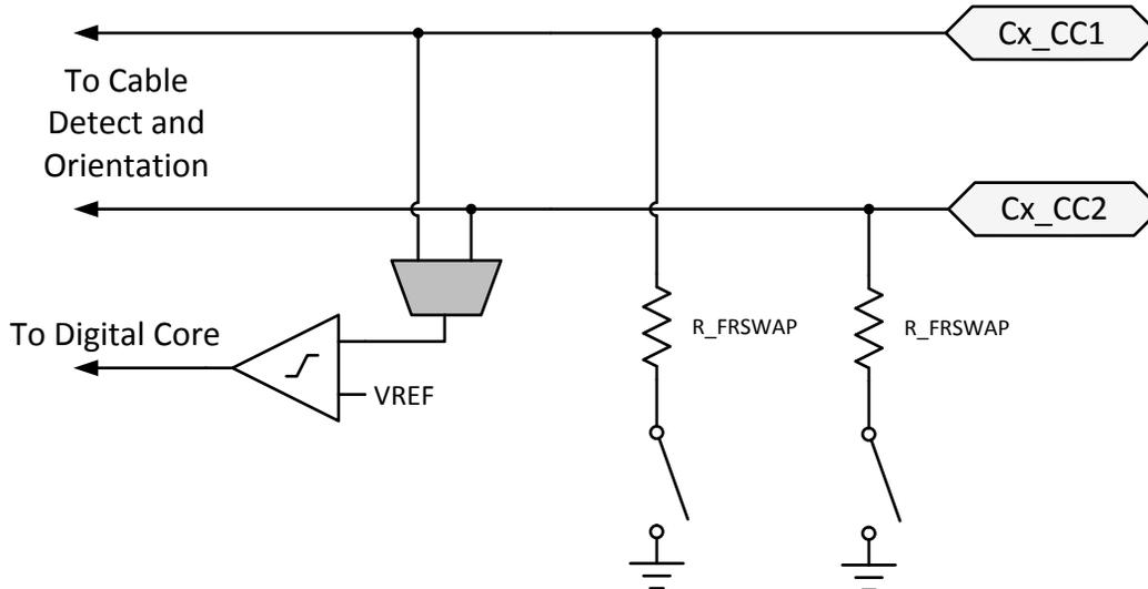
**Figure 8-15. Fast Role Swap Detection and Signaling**
