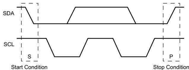
**Figure 8-23. I<sup>2</sup>C Definition of Start and Stop Conditions**
