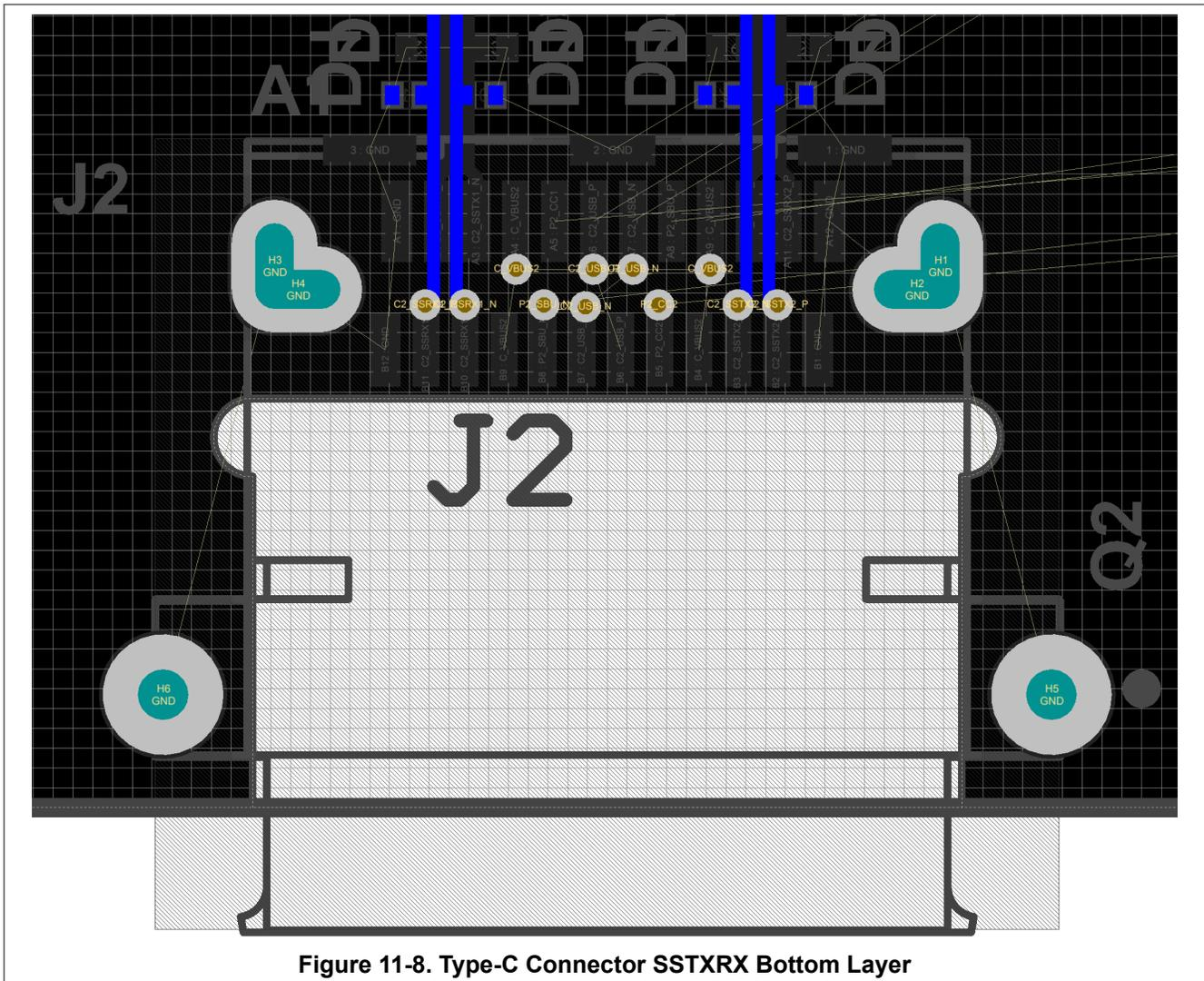
Figure 11-8. Type-C Connector SSTXRX Bottom Layer
