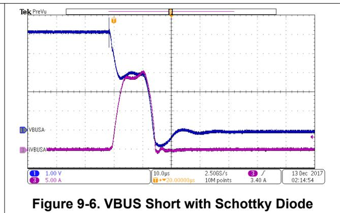
Figure 9-6. VBUS Short with Schottky Diode
