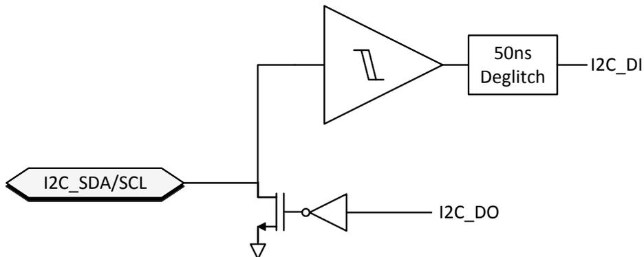
**Figure 8-20. I<sup>2</sup>C Buffer**
