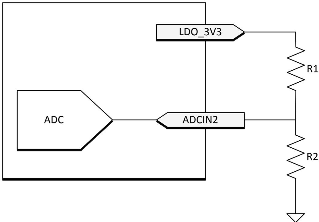
**Figure 8-29. I<sup>2</sup>C Address Divider**
