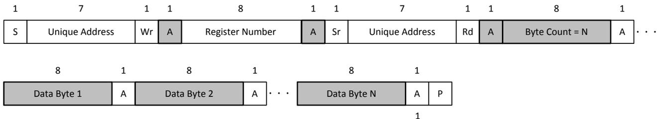
**Figure 8-27. I<sup>2</sup>C Unique Address Read Register Protocol**
