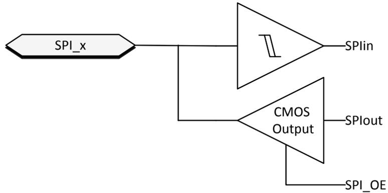
**Figure 8-21. SPI Buffer**
