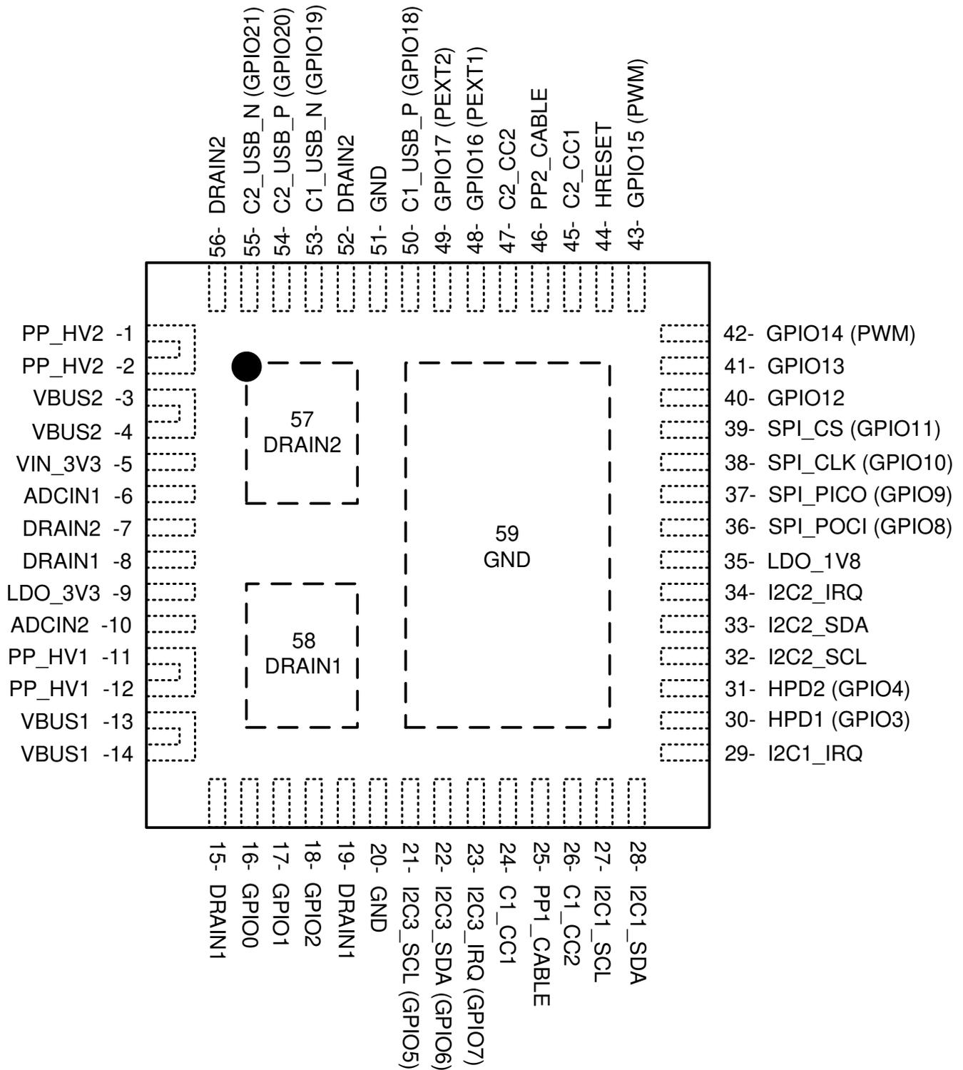
Figure 5-1. RSH Package 56-Pin QFN Top View
