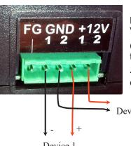
FG = Frame Ground (Do Not Connect to V-)
