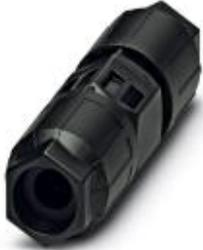
Conductor connectors, QUICKON connection, No. of pos.: 3+PE, 0.5 mm<sup>2</sup> ... 1.5 mm<sup>2</sup>, 690 V, 17.5 A, black, With two QUICKON nuts, Cable diameter: 4 mm ... 9 mm
