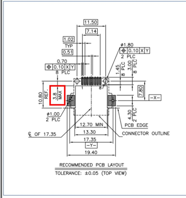
Distance between mounting hole position and mid mount edge will be 1.90mm MAX
