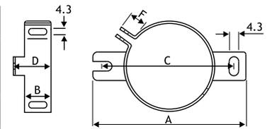
When using mounting clamps, care should be taken not to obscure any safety vent in the can. Delivered without bolts and nuts for mounting.
