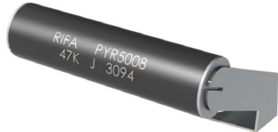
The PYR resistors are wire wound on a ceramic core and coated with high temperature silicone. The mounting brackets are made of stainless steel and connected by two point spot welding.
