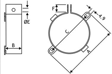
\*PYC clamps are for PEH169 and PEH200 capacitors only. Diameters include plastic insulation.
