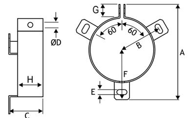
When using mounting clamps, care should be taken not to obscure any safety vent in the can. Delivered without bolts and nuts for mounting.
