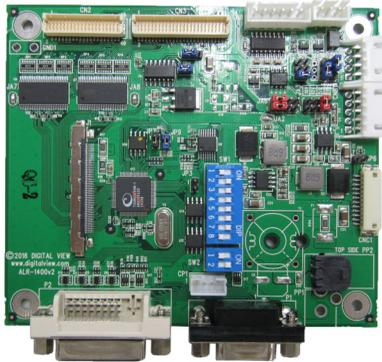
The HE-1400v2 is a compact LCD controller supporting LCD panels up to 1440 x 900 resolution with TTL and LVDS connection
