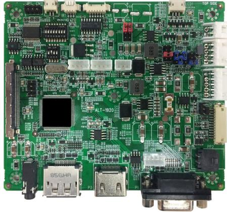
The ALT-1920 is a compact controller for LCD panels up to 1920 x 1200 with HDMI, Displayport & ARGB inputs
