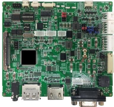
The HLT-1920 is a compact controller for LCD panels up to 1920 x 1200 with HDMI, Displayport & ARGB inputs
