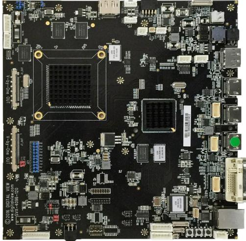
The SVX-4096-120 is a full function controller supporting 60Hz and 120Hz LCD panels up to 4096 x 2160 resolution
