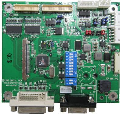
The ALR-1400v2 is a compact LCD controller supporting LCD panels up to 1440 x 900 resolution with TTL and LVDS connection
