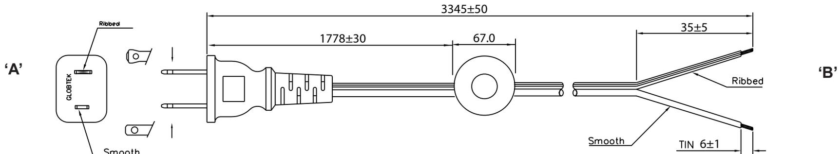
PUSHBUTTON SWITCH, Ø 67 mm WITH 23 mm BOTTOM,
