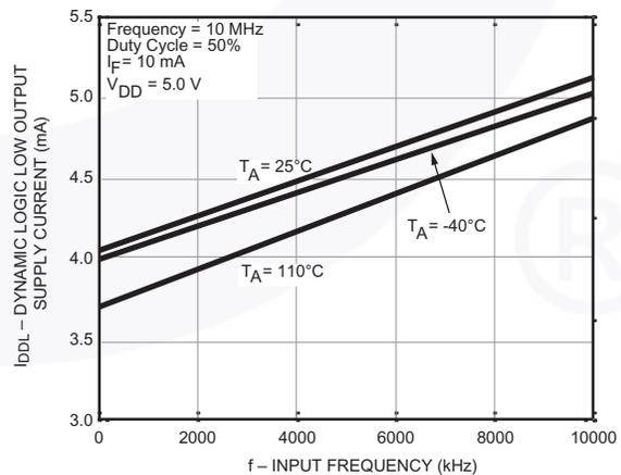
**Figure 7. Dynamic Logic Low Output Supply Current vs. Input Frequency (V<sub>DD</sub> = 5.0V)**
