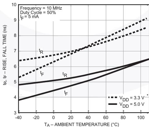
**Figure 12. Rise and Fall Time vs. Ambient Temperature**
