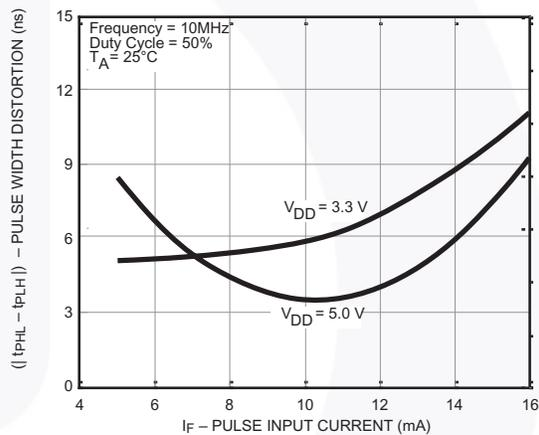
**Figure 11. Pulse Width Distortion vs. Pulse Input Current**
