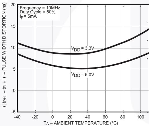
**Figure 10. Pulse Width Distortion vs. Ambient Temperature**
