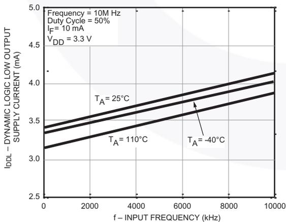
**Figure 6. Dynamic Logic Low Output Supply Current vs. Input Frequency (V<sub>DD</sub> = 3.3V)**
