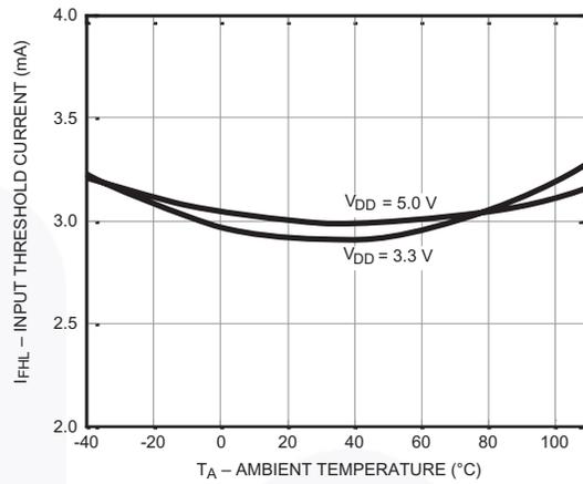
**Figure 3. Input Threshold Current vs. Ambient Temperature**
