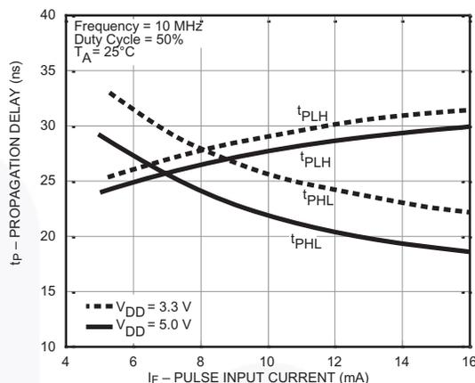
**Figure 9. Propagation Delay vs. Pulse Input Current**
