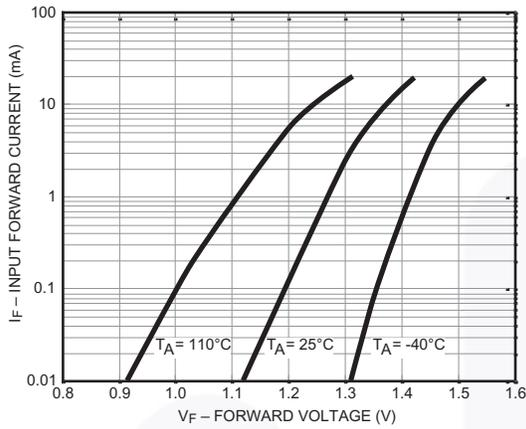
**Figure 2. Input Forward Current vs. Forward Voltage**
