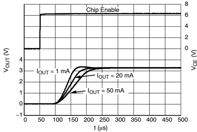
Figure 39. Start-up, 3.3 V Version,  $V_{\text{IN}} = 6.3 \text{ V}$
