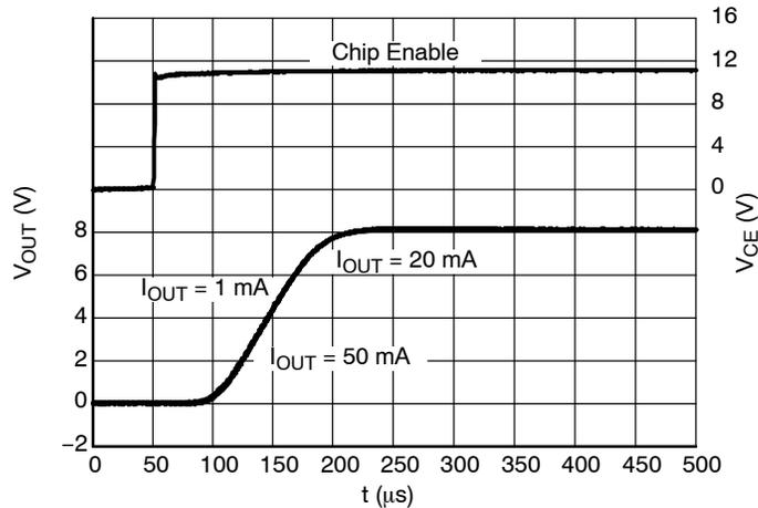
Figure 40. Start-up, 8.0 V Version,  $V_{\text{IN}} = 11.0 \text{ V}$
