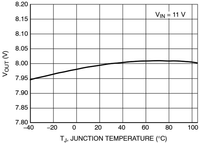
**Figure 11. Output Voltage vs. Temperature, 8.0 V Version**
