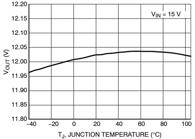
**Figure 12. Output Voltage vs. Temperature, 12 V Version**
