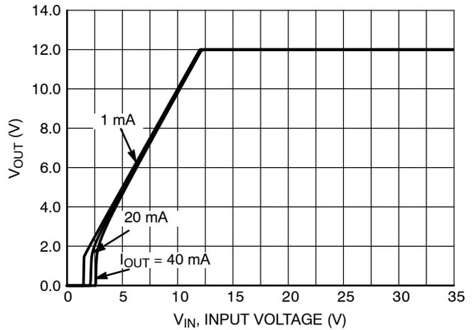
Figure 18. Output Voltage vs. Input Voltage, 12 V Version
