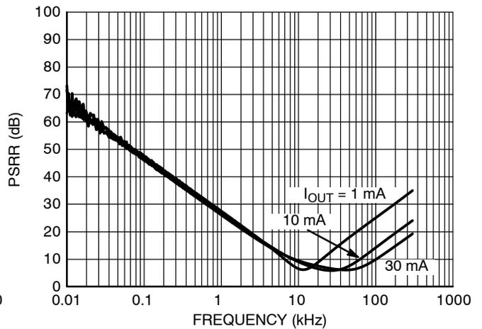
Figure 20. PSRR, 3.3 V Version,  $V_{IN} = 6.3 V$
