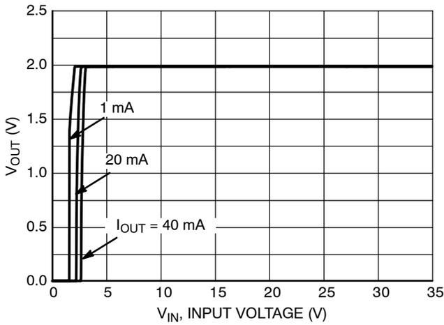
Figure 15. Output Voltage vs. Input Voltage, 2.0 V Version
