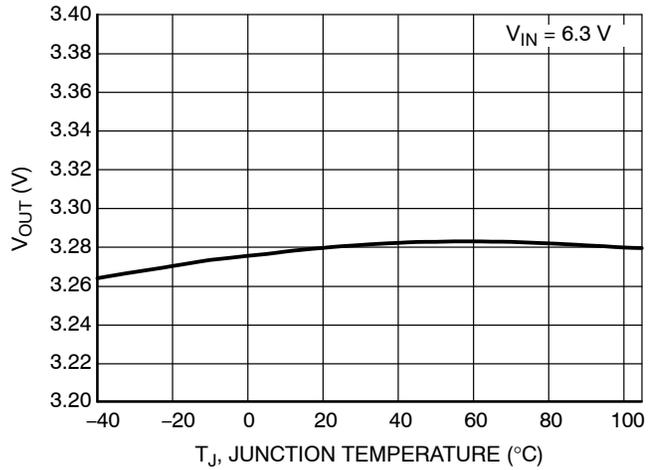
**Figure 10. Output Voltage vs. Temperature, 3.3 V Version**
