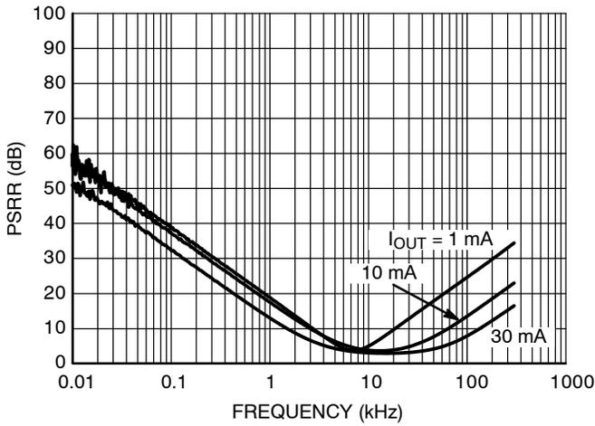
Figure 21. PSRR, 3.3 V Version,  $V_{IN} = 6.3 \text{ V}$
