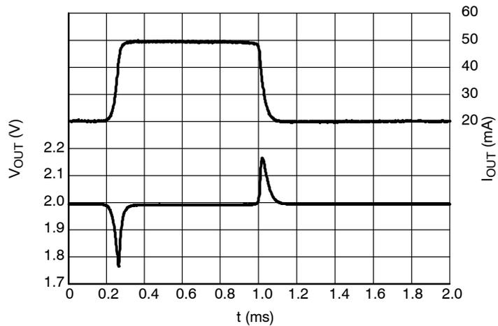
**Figure 34. Load Transients, 2.0 V Version,
