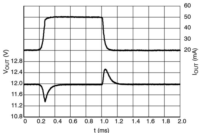
**Figure 37. Load Transients, 12.0 V Version,
