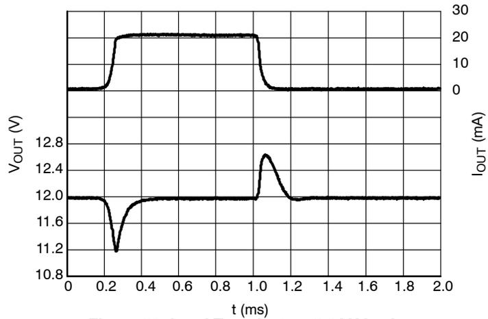
**Figure 33. Load Transients, 12.0 V Version,
