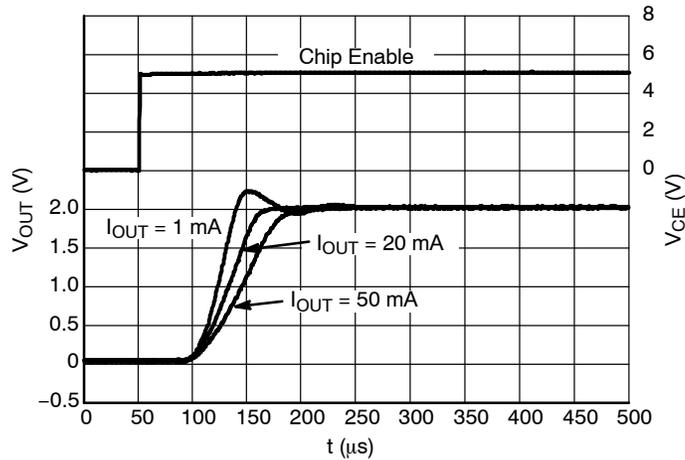
Figure 38. Start-up, 2.0 V Version,  $V_{\text{IN}} = 5.0 \text{ V}$
