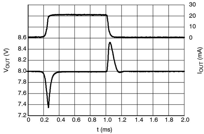
**Figure 32. Load Transients, 8.0 V Version,
