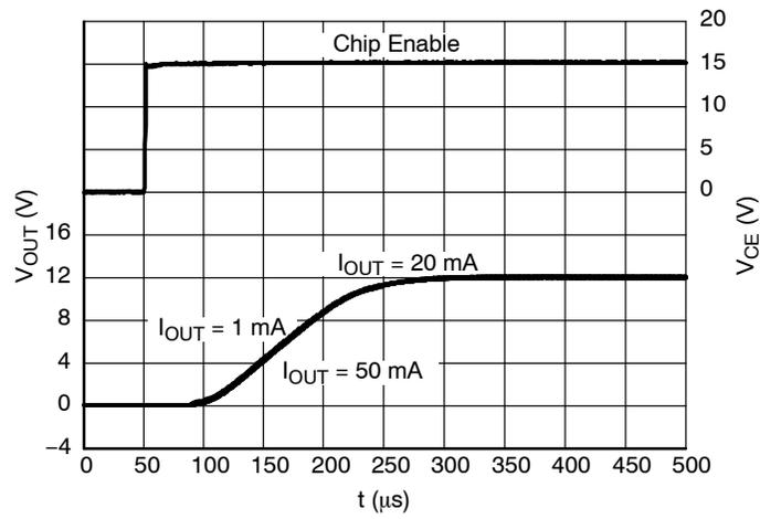
Figure 41. Start-up, 12.0 V Version,  $V_{IN} = 15.0 \text{ V}$
