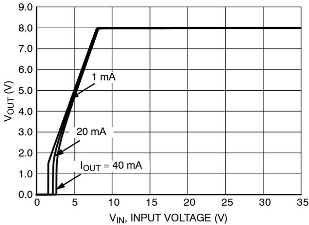
Figure 17. Output Voltage vs. Input Voltage, 8.0 V Version
