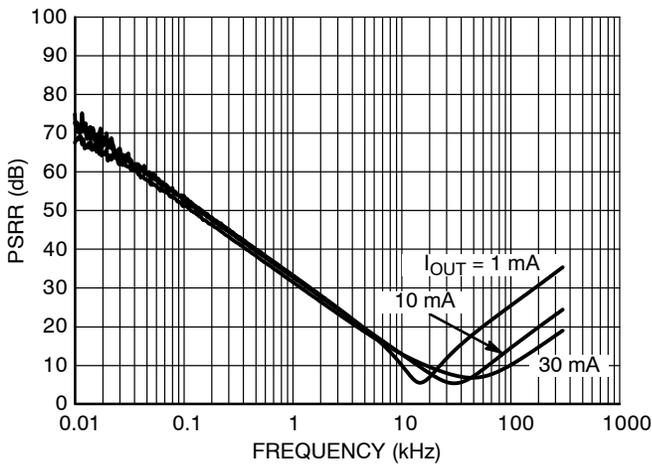
Figure 19. PSRR, 2.0 V Version,  $V_{IN} = 5.0 V$
