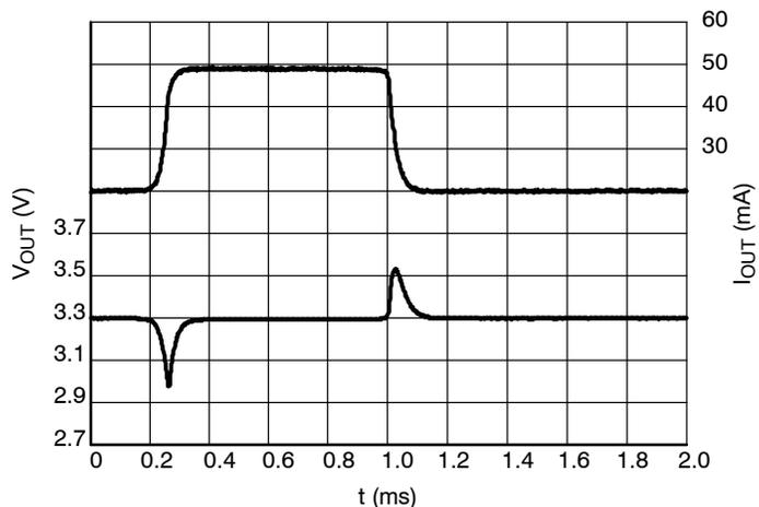
**Figure 35. Load Transients, 3.3 V Version,
