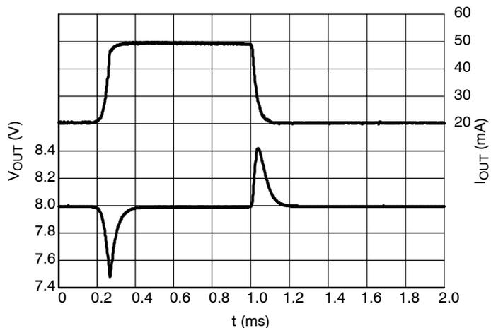
**Figure 36. Load Transients, 8.0 V Version,
