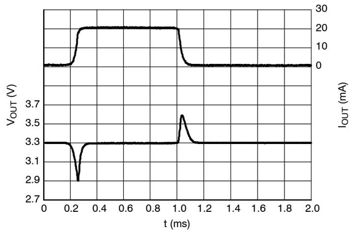
**Figure 31. Load Transients, 3.3 V Version,
