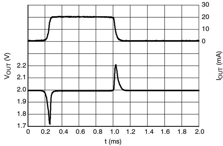
**Figure 30. Load Transients, 2.0 V Version,
