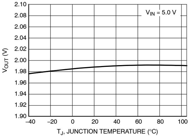
**Figure 9. Output Voltage vs. Temperature, 2.0 V Version**
