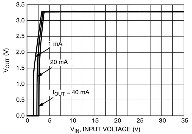
Figure 16. Output Voltage vs. Input Voltage, 3.3 V Version
