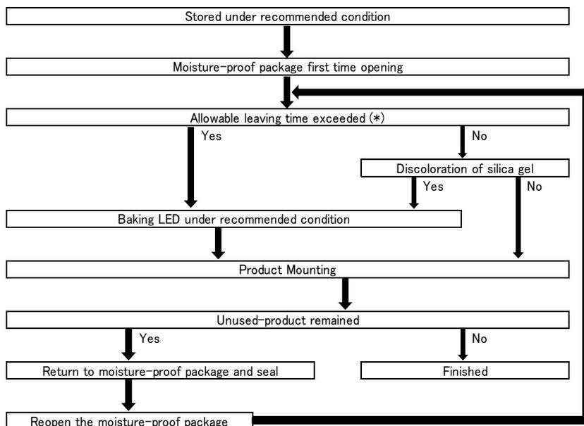
Allowable leaving time means the maximum allowable leaving time after opening package, which depends on each LED type. The allowable leaving time should be calculated from the first opening of package to the time when soldering process is finished. When judging if the allowable leaving time has exceeded or not, please subtract the soldering time. The allowable leaving time after reopening should be calculated from the first opening of package, or from the time when baking process is finished.
