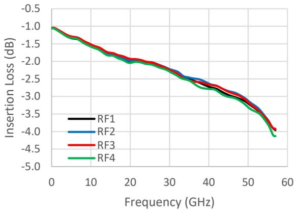
**RFC to RF1 Insertion Loss over Temperature<sup>11</sup>**
