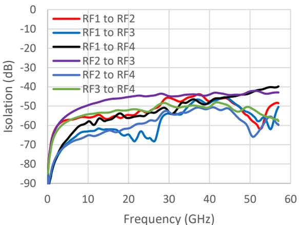
**Isolation between RF1 to RF4, RFC to RF4 On<sup>11</sup>**
