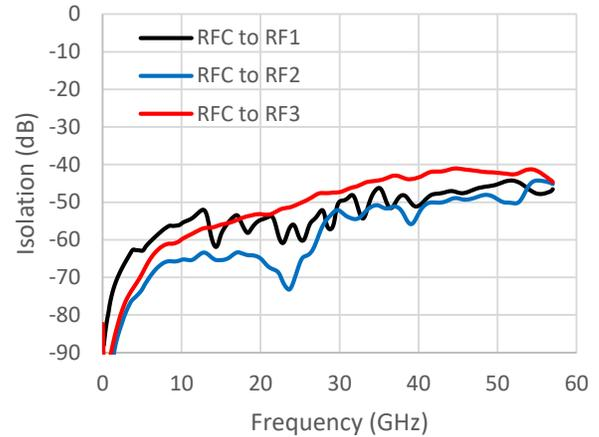
**RFC to RF1 / RF3 / RF4 Isolation, RFC to RF2 On<sup>11</sup>**
