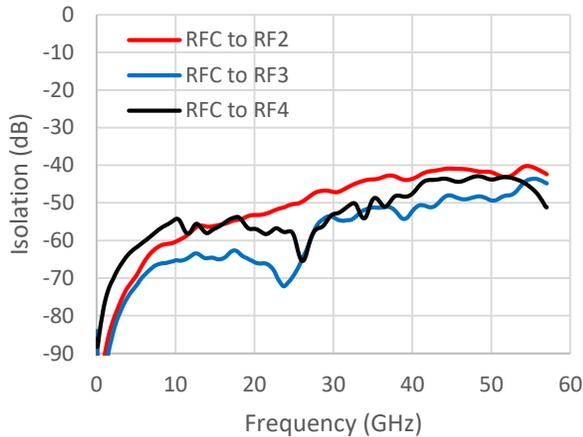
**RFC to RF1 / RF2 / RF3 Isolation, RFC to RF4 On<sup>11</sup>**
