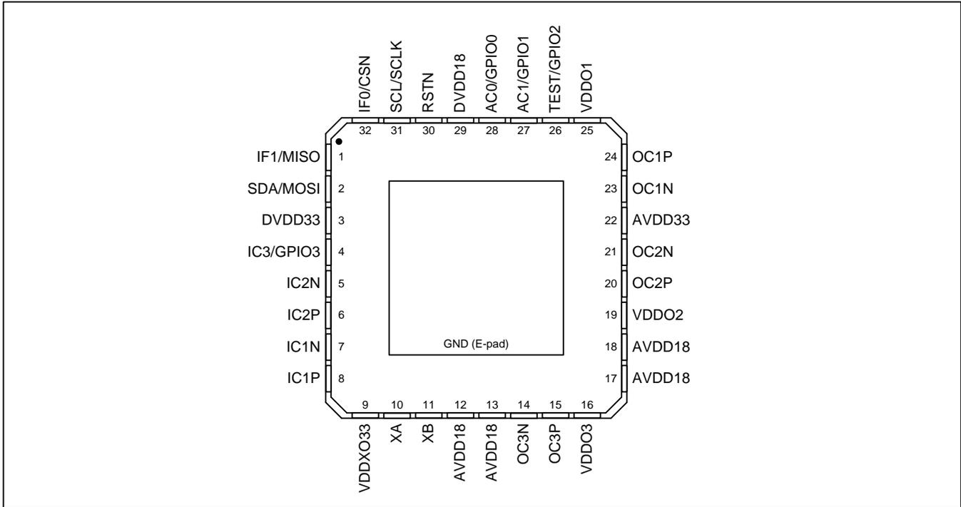
**Figure 2 - Pin Diagram**
